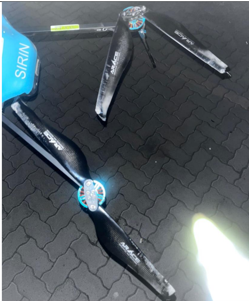
Figure 3: The damaged propeller, motor and landing gear assembly. (Source: Operator)
