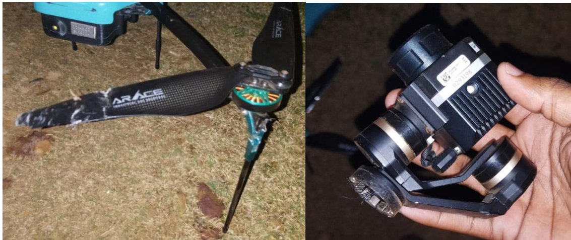
Figure 2: The damaged propeller (left) and gimbal (right). (Source: Operator)
