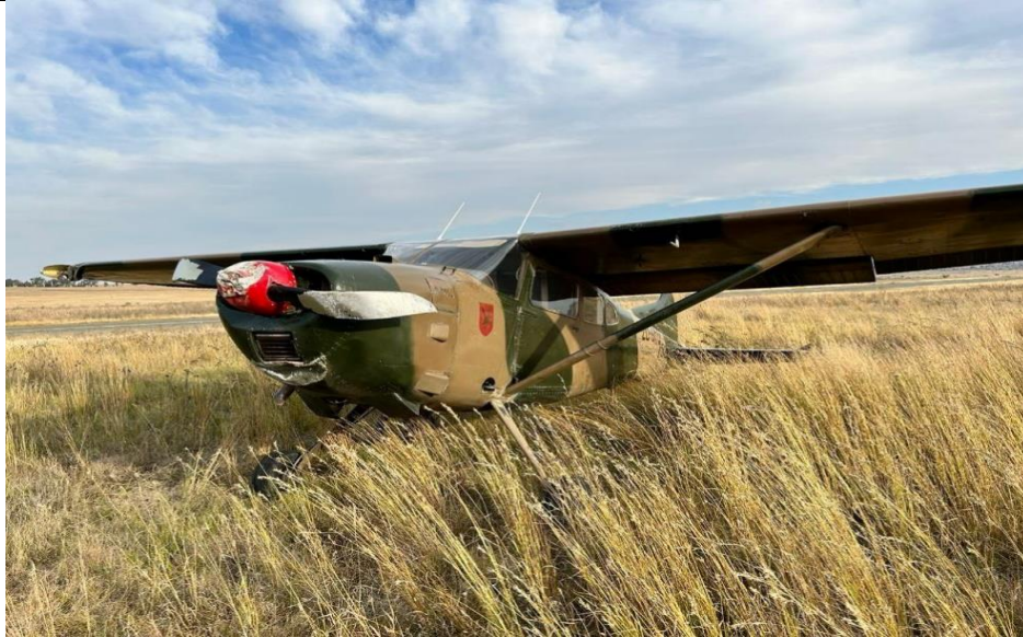
Figure 2: The aircraft with damaged propeller blades and spinner. (Source: Pilot)
