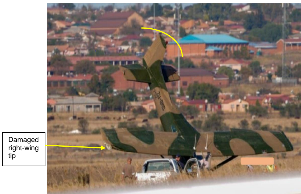
Figure 1: The aircraft post-accident with the tail lifted, indicated by the yellow arch. (Source: Pilot)
