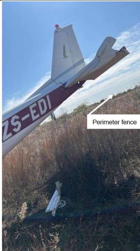
Figure 3: The damaged perimeter fence and the broken nose gear assembly. (Source: Operator)
