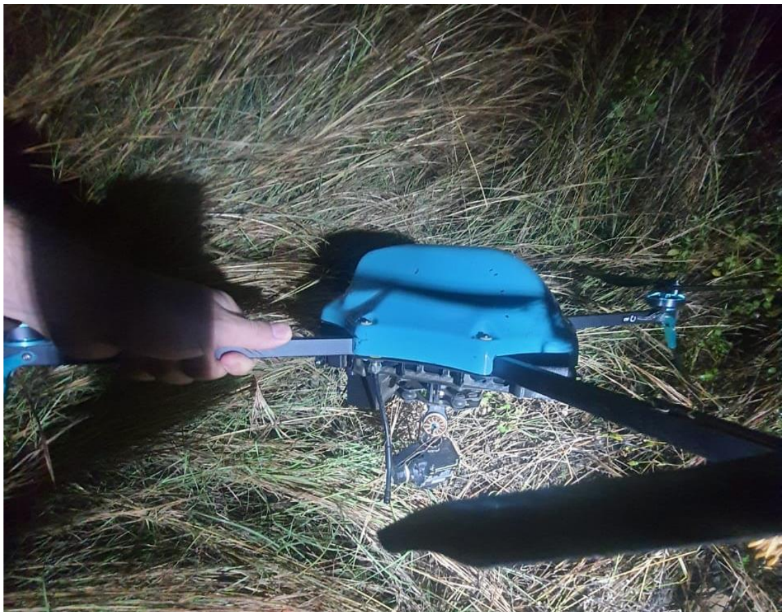
Figure 2: Damaged camera and skid. (Source: Operator)
