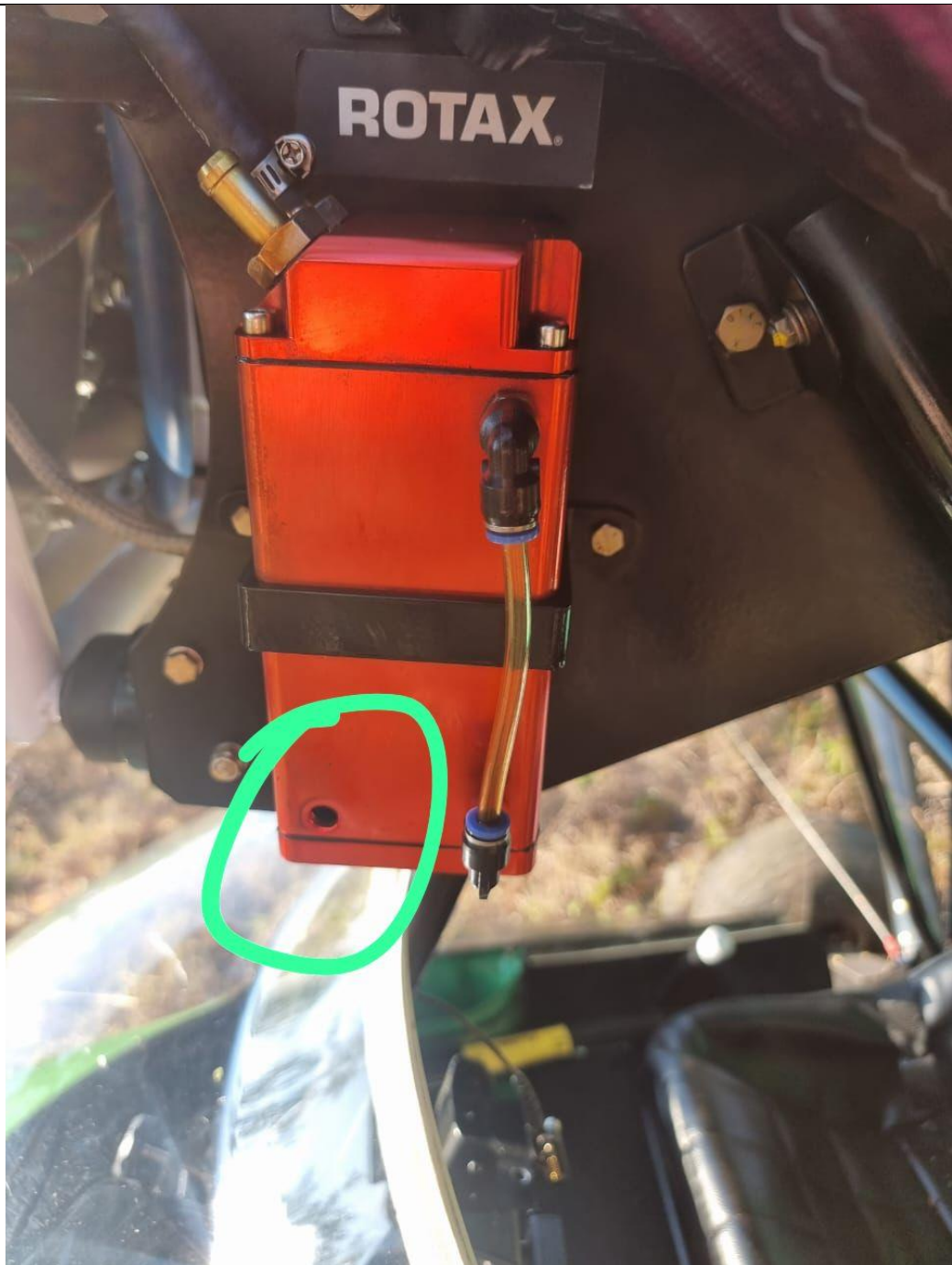
Figure 5: The oil breather container with the drain plug missing. (Source: Pilot)
