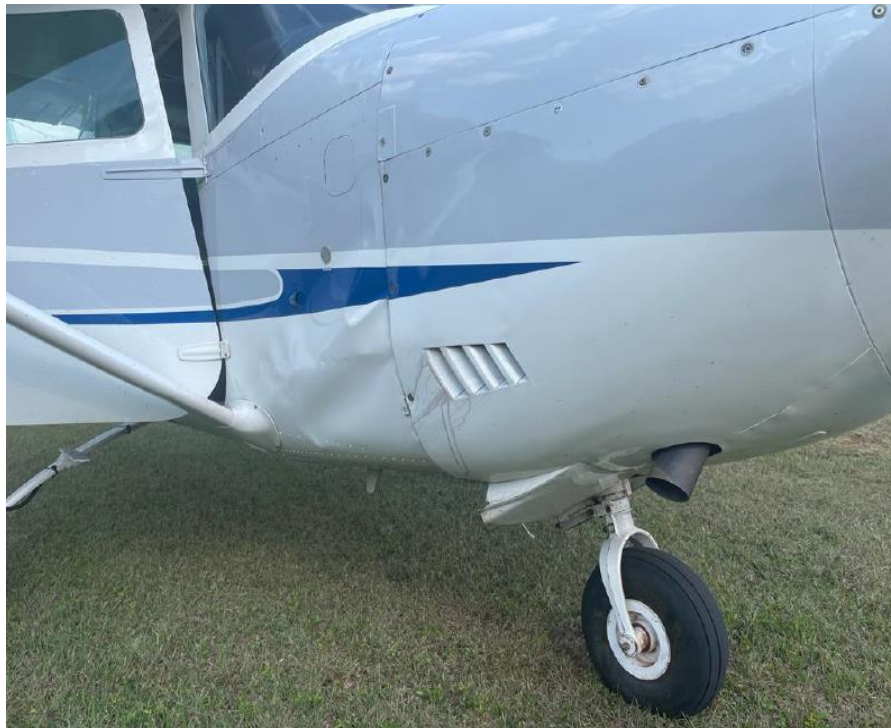
Figure 2: The damaged airframe. (Source: Operator)
