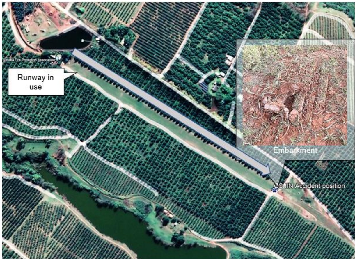
Figure 3: The airstrip (white arrow indicating the direction of flight) and the embankment on the runway end where the aircraft impacted the ground just before it careered onto the road. (Source: Google map)
