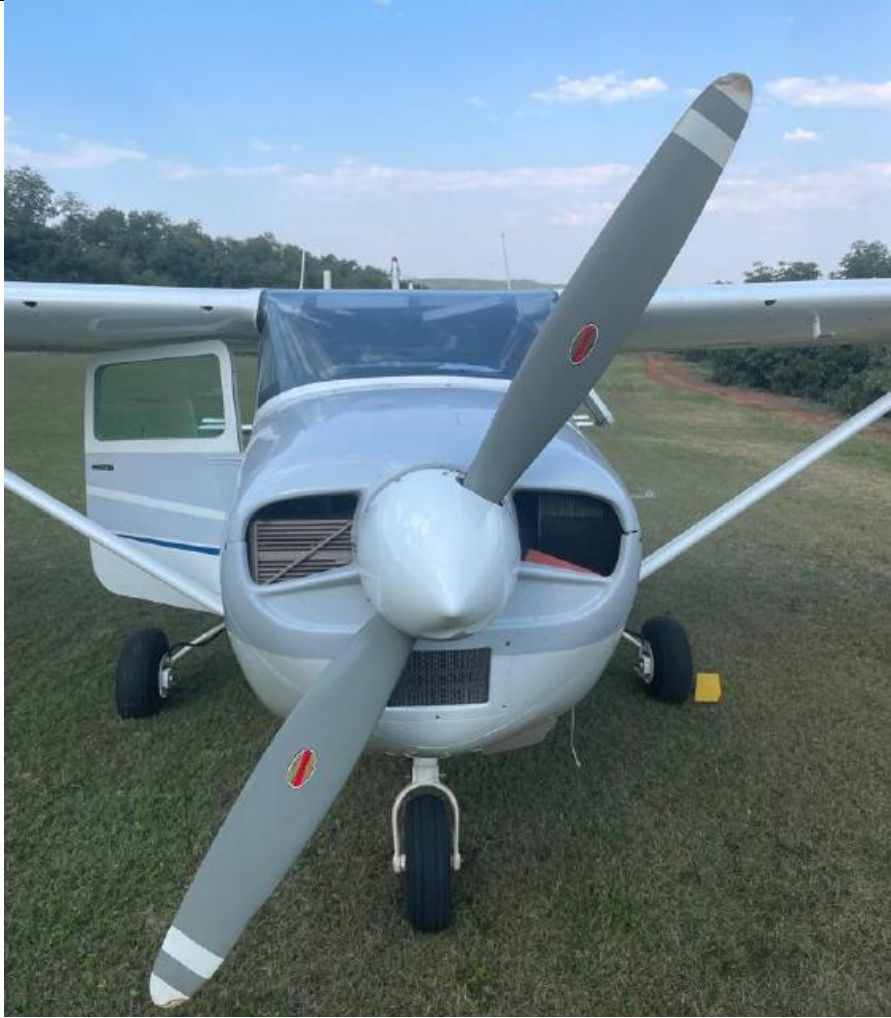
Figure 1: The damaged propeller blade tips. (Source: Operator)
