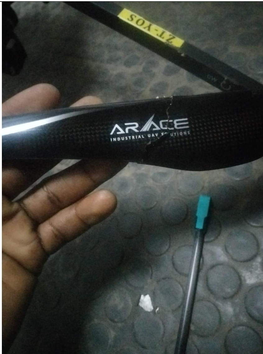
Figure 3: The damaged propeller. (Source: Operator)
