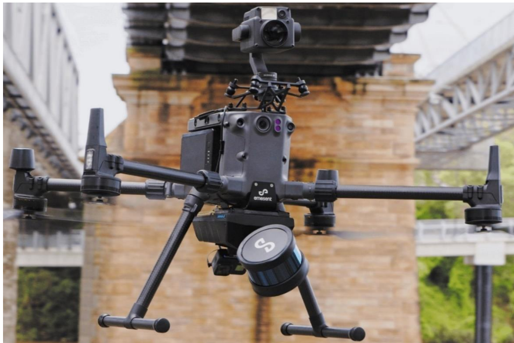
Figure 2: An example of a DJI Matrice 300 similar to the one that was involved in an accident. (Source: https://enterprise.dji.com/ecosystem/hovermap )
