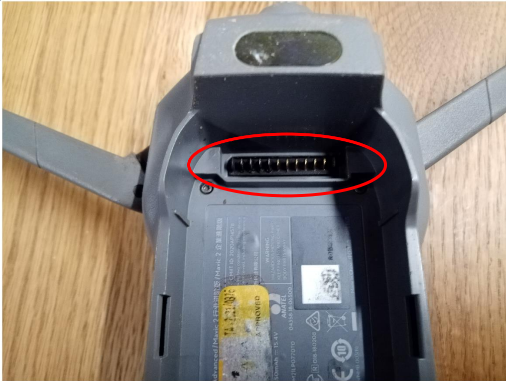
Figure 4: Red circle shows the burnt battery terminals. (Source: Operator)
