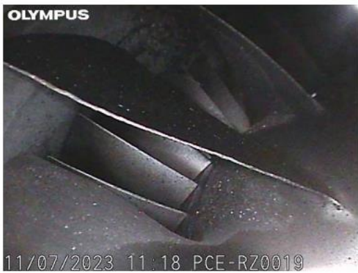
1 st stage compressor blade condition with light levels of erosion and oil wetness observed. Foreign debris observed.
