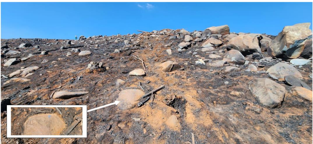
Figure 5: A blue paint mark on the rock that the aircraft's hopper impacted.
