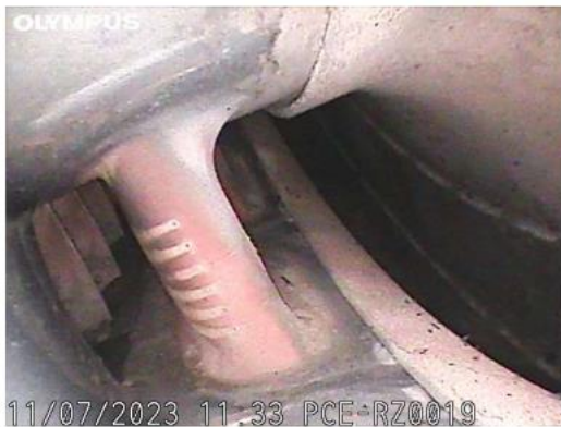
C.T. vane condition with light thermal coating deterioration, dirt build-up and light cracking
