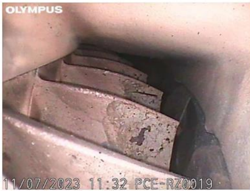
C.T. blade and segment condition with light erosion and dust build-up observed. Foreign debris observed in CT. area.
