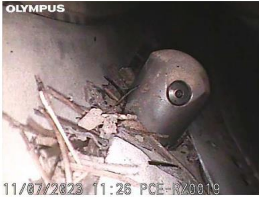
Combustion chamber with light thermal erosion and foreign debris observed.
