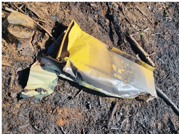
Figure 12: The right-side aileron with the trim tab missing. Figure 13: Shows the left-side aileron with the trim tab still attached.
