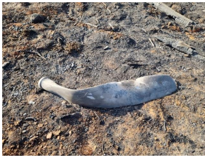
Figures 15, 16 and 17: Three of the five propeller blades were recovered at the accident site.
