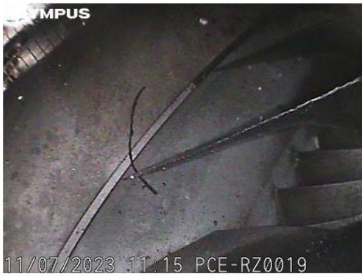
Compressor inlet housing condition with areas moderate coating deterioration and associated coating loss. Evidence of foreign debris observed (Grass, sand/dirt etc.).
