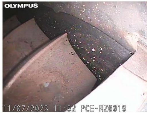
C.T. blade and segment condition with light erosion and dust build-up observed. Foreign debris observed in CT. area.
