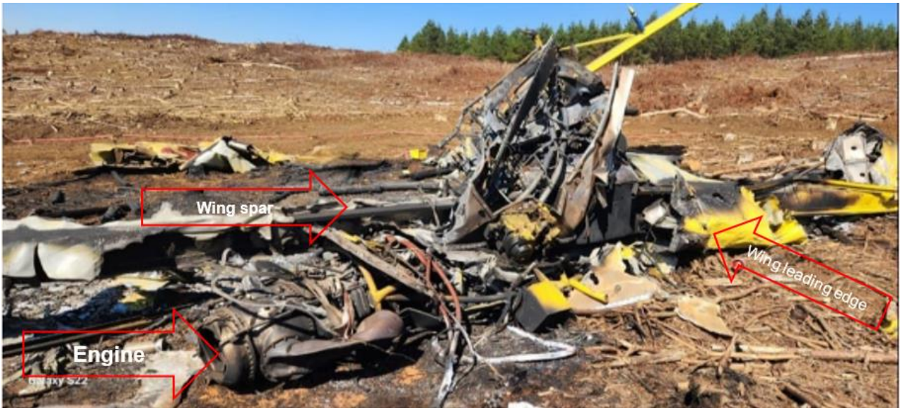
Figure 8: The front view of the main wreckage with damaged wings.
