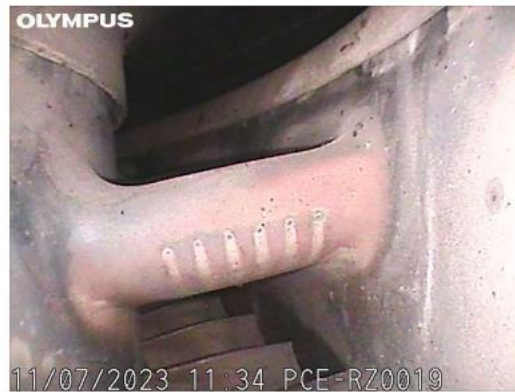
C.T. vane condition with light thermal coating deterioration, dirt build-up and light cracking
