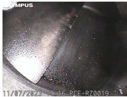
1 st stage compressor blade condition with light levels of erosion and oil wetness observed. Foreign debris observed.
