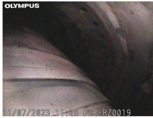
Combustion chamber with light thermal erosion and foreign debris observed.
