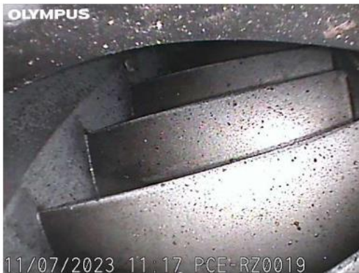
1 st stage stator with light L.E. erosion and dirt build-up observed. 2 nd stage comp. blade condition with light L.E. erosion observed. Foreign debris observed in 2 nd stg. compressor area.
