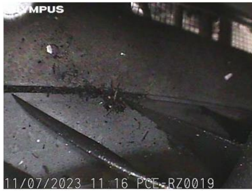
Compressor inlet housing condition with areas moderate coating deterioration and associated coating loss. Evidence of foreign debris observed (Grass, sand/dirt etc.).
