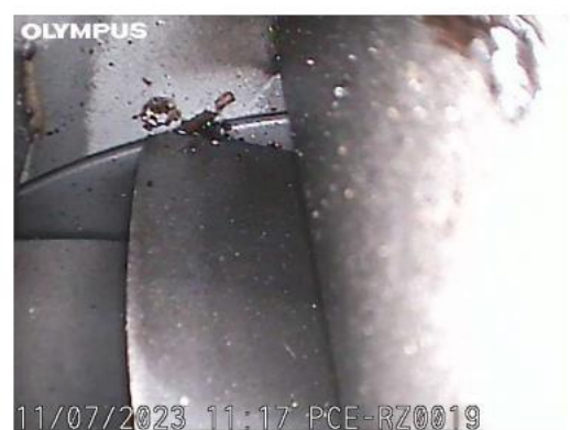
1 st stage stator with light L.E. erosion and dirt build-up observed. 2 nd stage comp. blade condition with light L.E. erosion observed. Foreign debris observed in 2 nd stg. compressor area.
