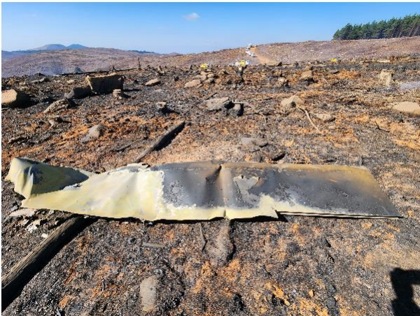
Figure 12: The right-side aileron with the trim tab missing. Figure 13: Shows the left-side aileron with the trim tab still attached.
