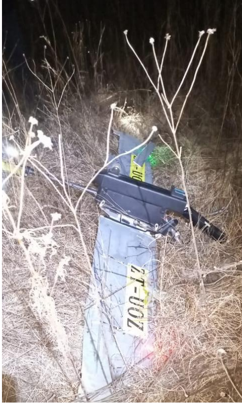
Figures 1 and 2: The UAS at the accident site in an inverted position with the right aileron separated (left); and damage on the UAS gimbal and front fuselage (right). (Source: Operator)
