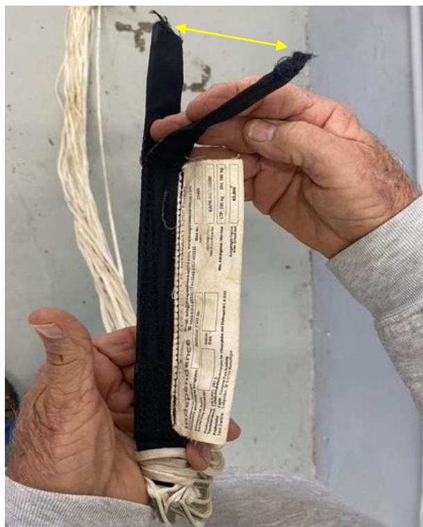
Figure 12: Paraglider 1 reserve strop that snapped.
