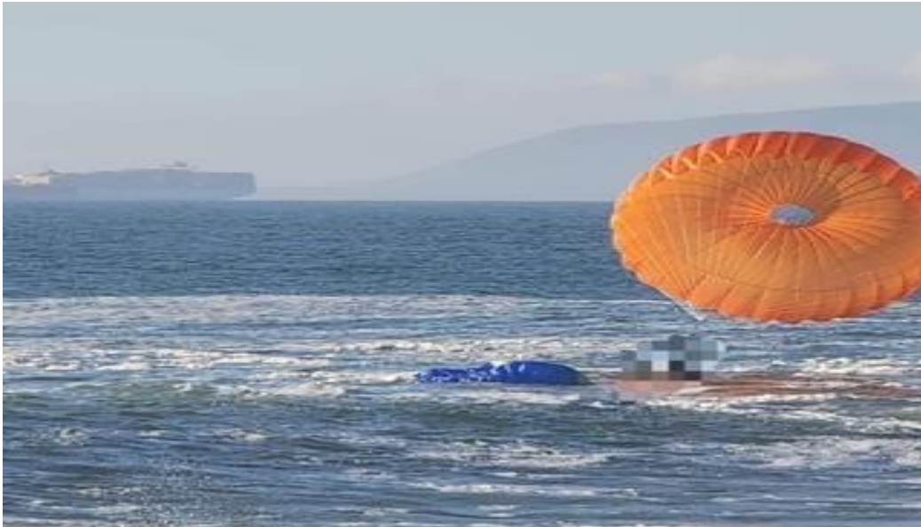
Figure 3: Paraglider 1's wing partially submerged (blue) in the ocean, and the deployed reserve parachute. (Source: Eyewitness mobile phone footage)
