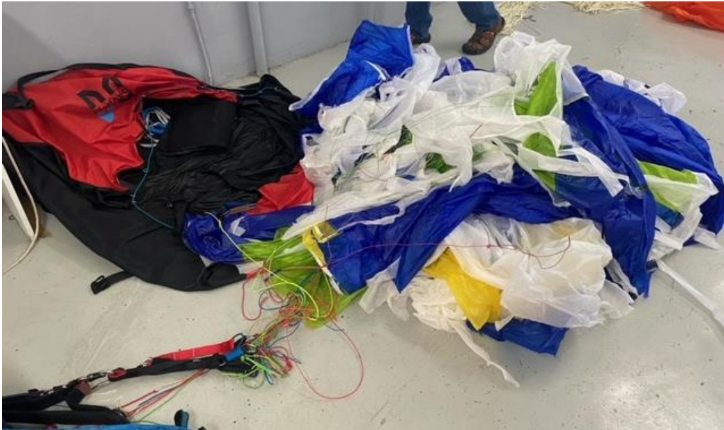
Figure 11: The torn wing fabric of Paraglider 1.
