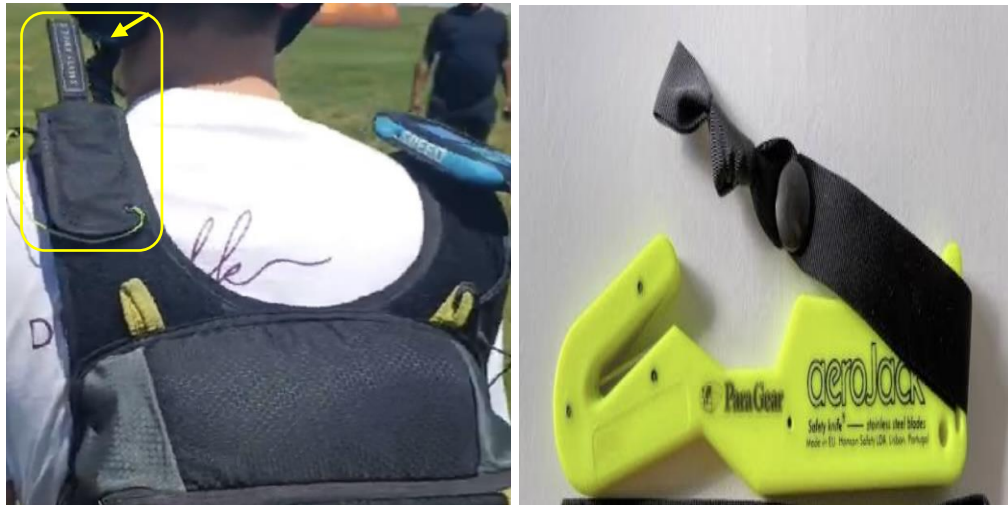
Figures 16 and 17: An illustration of the area where a hook knife is usually placed (left); hook knife (right). (Source: SAHPA)
