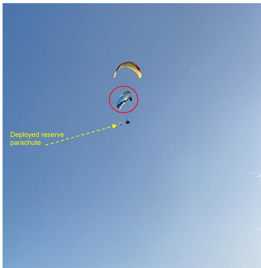
Figure 8: Video footage shows the wing of Paraglider 1 impacting Paraglider 2 occupants from bottom left-side (red circle). (Source: Eyewitness mobile phone footage)
