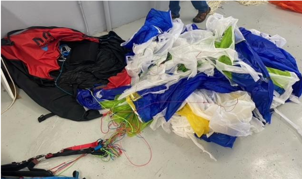
Figure 11: The torn wing fabric of Paraglider 1.
