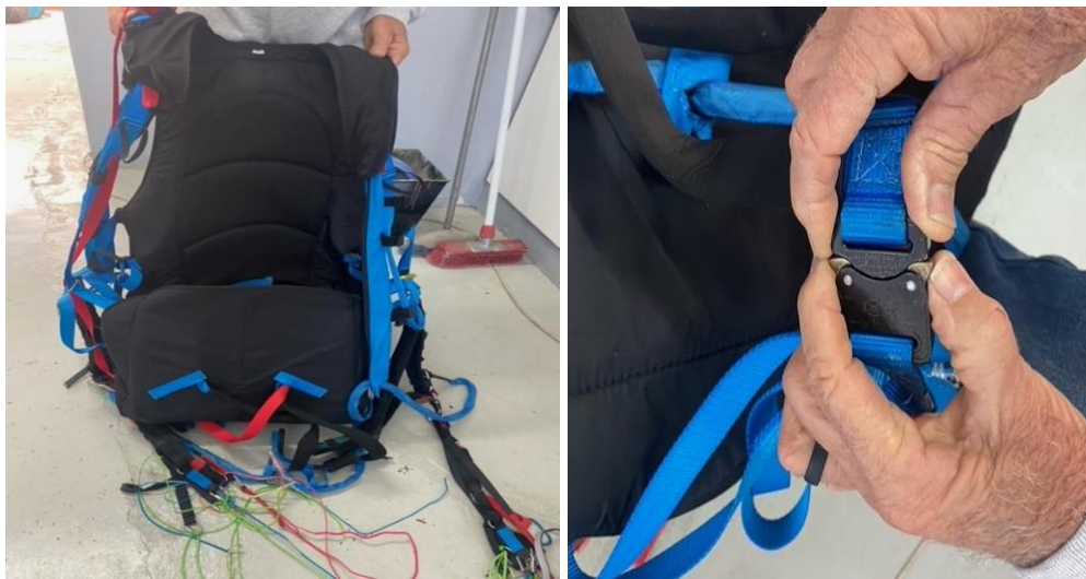
Figures 14/15: The flight instructor's seat (left) and its safety buckle/clip in a locked position (right).
