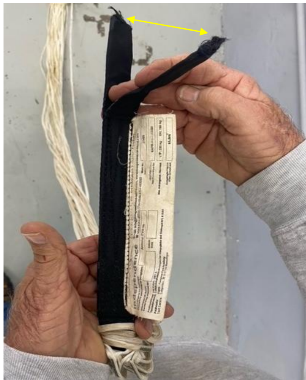
Figure 12: Paraglider 1 reserve stop that snapped.
