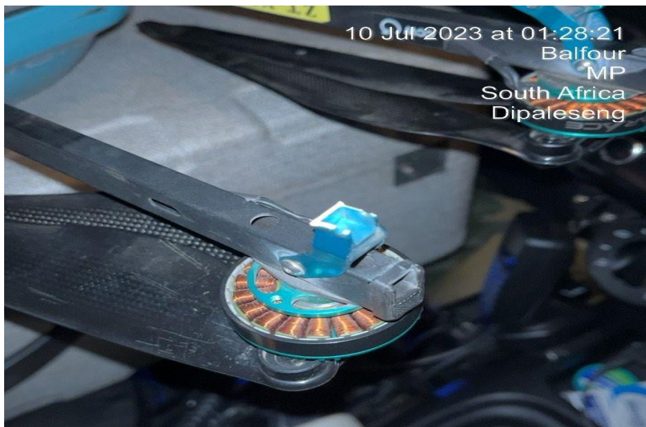
Figure 4: Damaged UAS landing gear. (Source: Operator)
