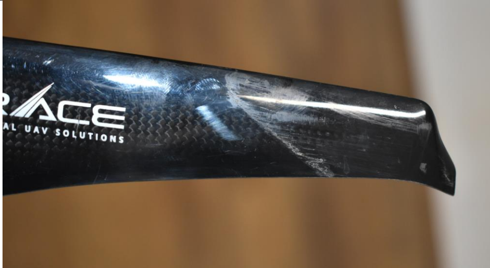
Figure 5: Scratch marks on the rotor blade. (Source: Operator)
