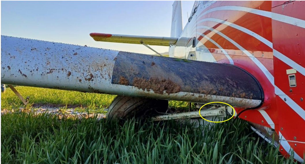
Figure 5: The front view of the broken right main gear. (Source: Operator)
