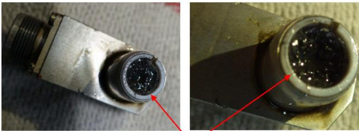
Figure 9: RGB Chip detector with arrows pointing to debris. (Source: Engine manufacturer)
