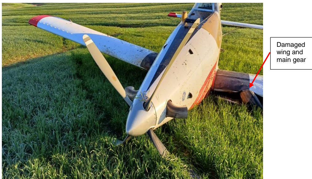
Figure 3: The front view of the aircraft at the accident site. (Source: Operator)
