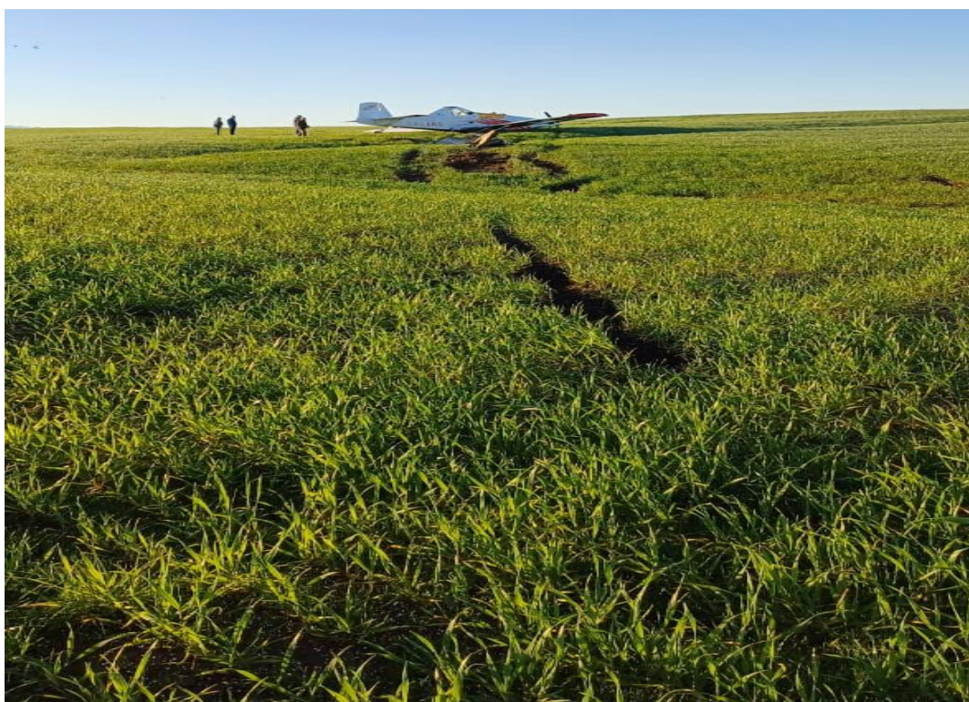
Figure 4: The path created by the aircraft's wheels in the wheat field. (Source: Operator)
