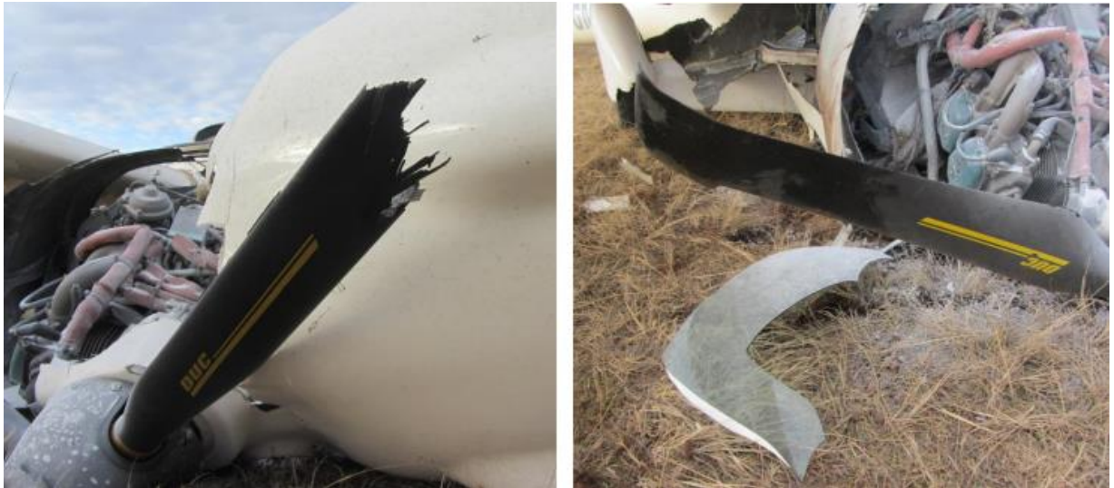
Figures 9 and 10: Damage sustained by the propeller blades.
