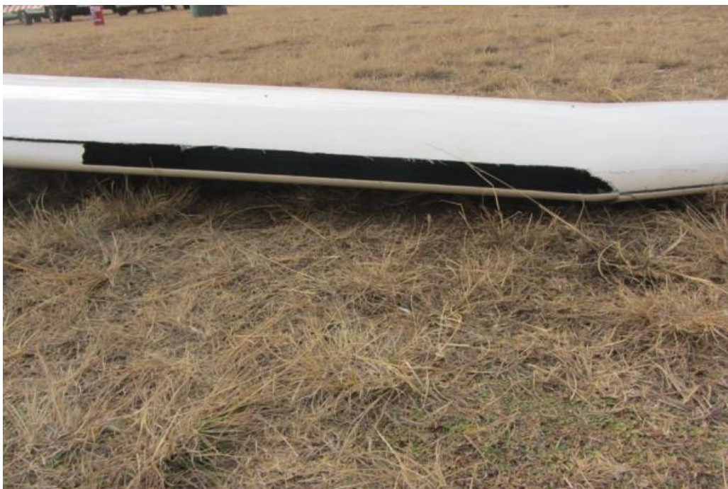
Figure 7: Damage on the right-side wing leading edge.
