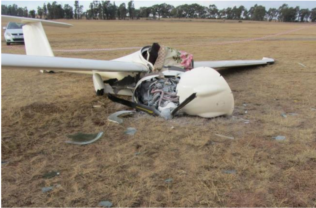
Figure 2: The damaged TMG after the accident.
