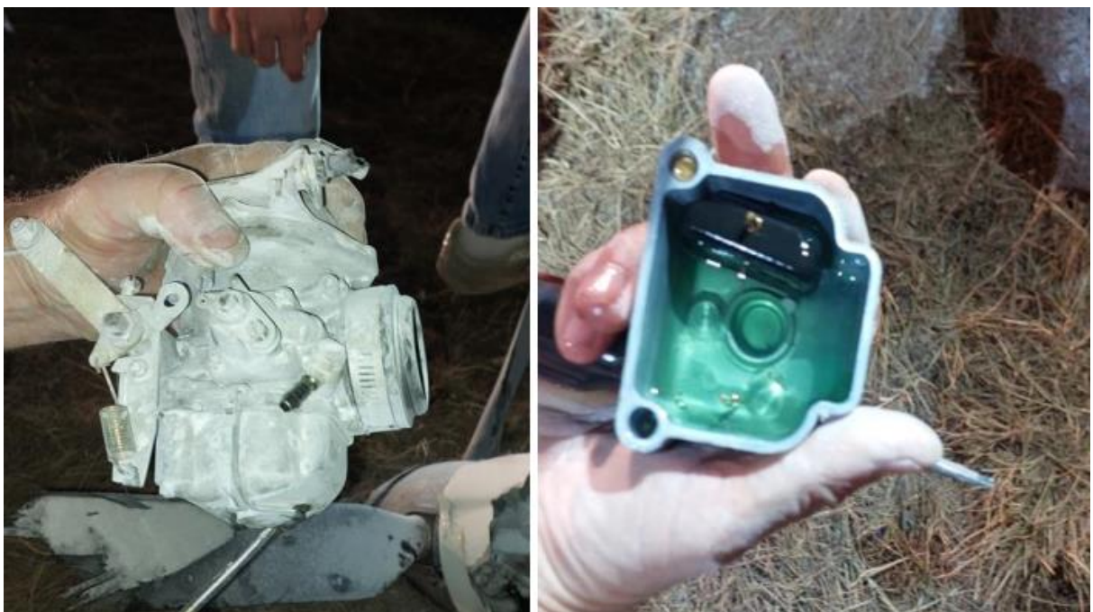
Figures 11 and 12: Carburettor (left) and bowl with fuel (right).
