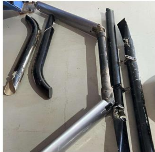
Figure 3: Broken left skid gear.
