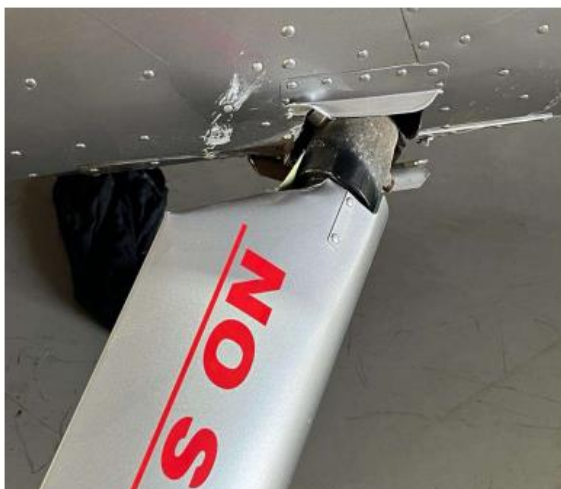
Figure 2: Damaged skid attachment.
