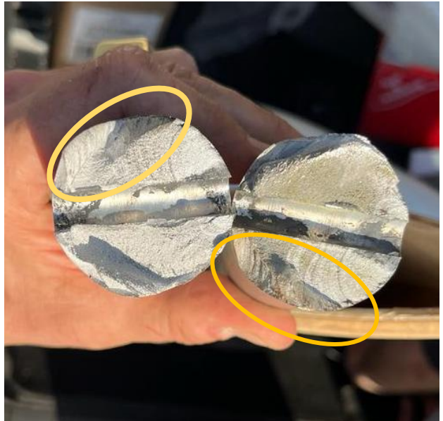
Figure 3: The right main landing strut that broke off during the landing roll. Figure 4: The yellow circles indicate a fatigue surface area which was not detected during maintenance. (Source: Operator)
