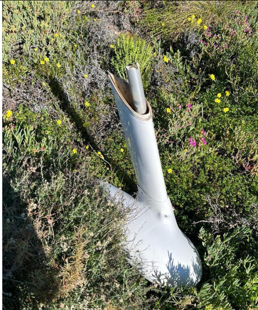
Figure 3: The right main landing strut that broke off during the landing roll. Figure 4: The yellow circles indicate a fatigue surface area which was not detected during maintenance. (Source: Operator)
