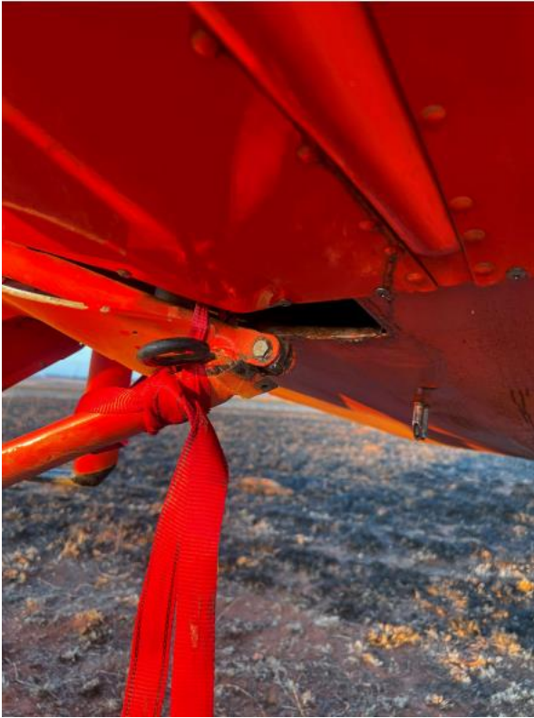
Figure 3: Right-side landing gear with the broken Hydrasorb shock absorbers. In the picture, a rope is tied to prevent the collapse of the landing gear.
