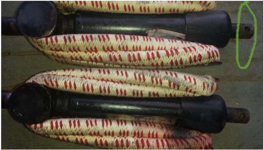
Figure 8: Example of an assembled Hydrasorb shock absorber with bungies; a circle indicates a failed mounting boss.
