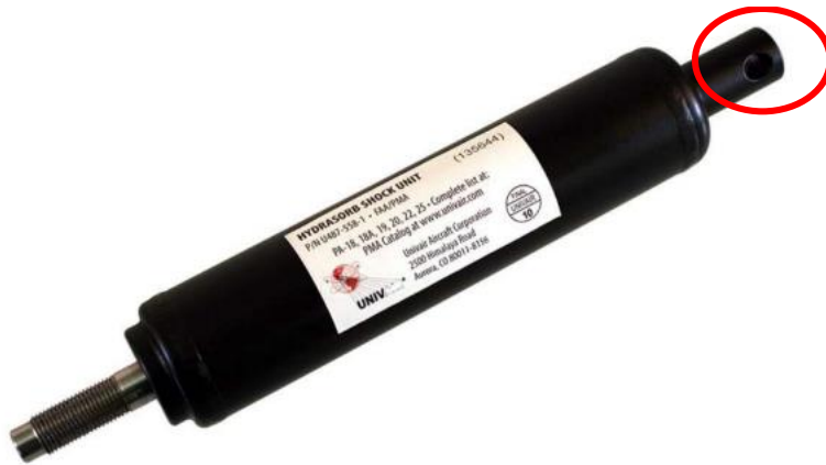
Figure 5: Mounting boss where it broke off.
