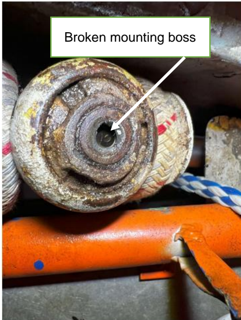
Figure 5: Mounting boss where it broke off.
