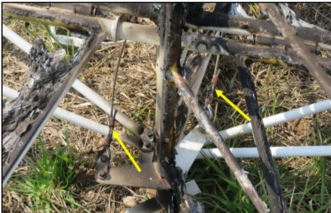
Figure 10: The two rudder cables were secured on both sides of the rudder attachments.
