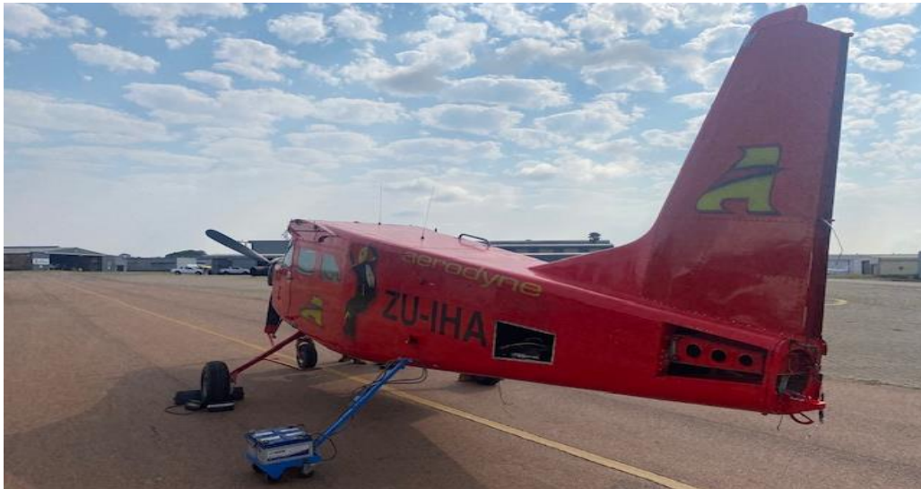
Figure 11: The aircraft during the engine ground run.
