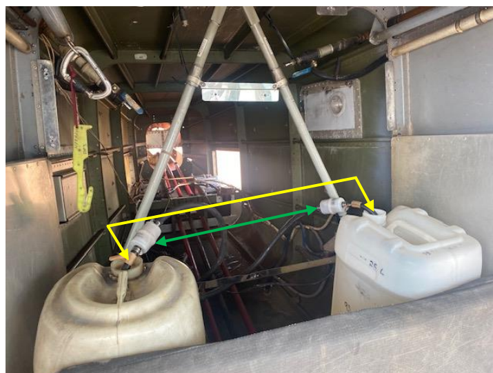
Figure 10: Fuel pipes dipped into the two 25l containers with fuel filters visible on each side.
