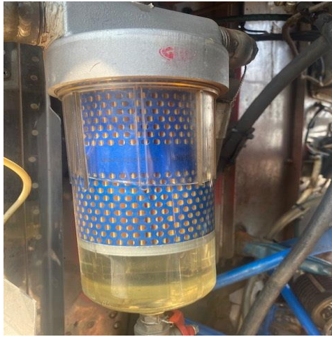
Figure 9: The engine main fuel filter. (Source – Aircraft Maintenance Organisation)
