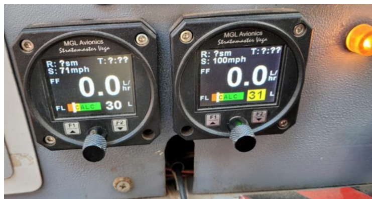
Figure 8: The fuel gauges showing the amount of fuel in the tanks post-accident. (Source: Pilot)
