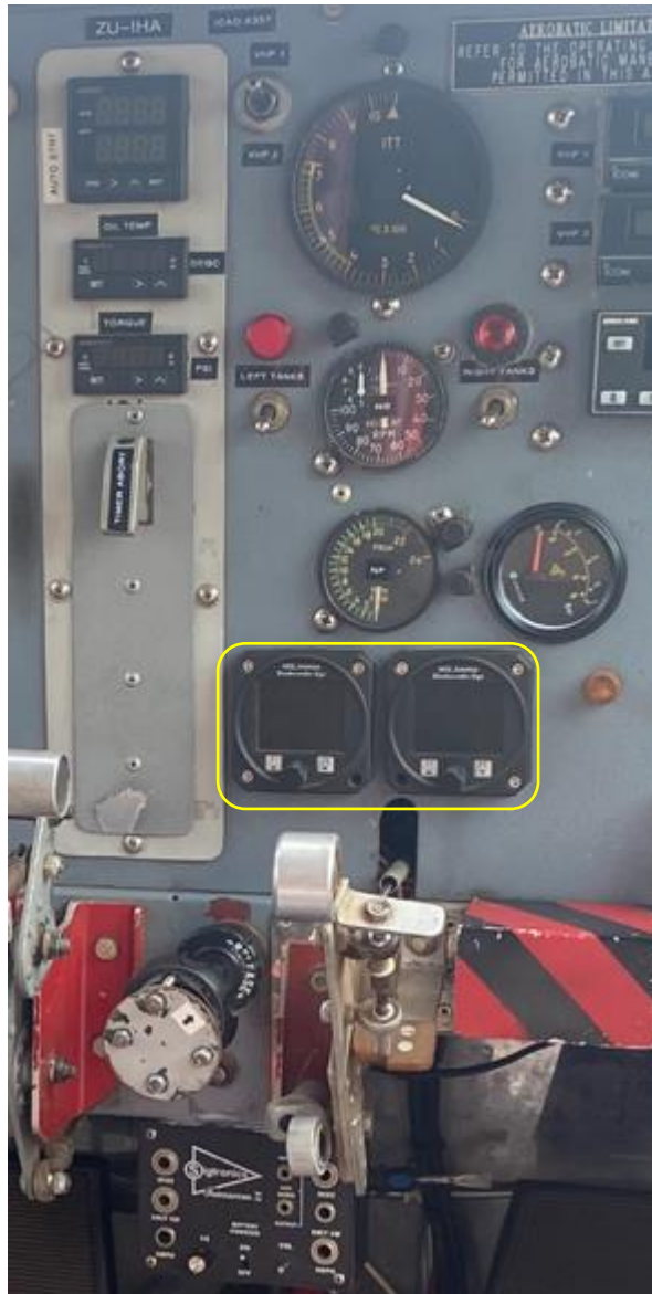
Figure 4: The two digital fuel gauges (yellow window) on the instrument panel.
