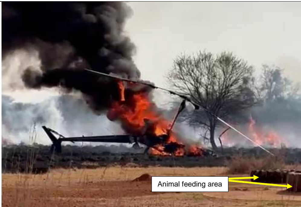
Figure 2: A still picture extracted from a video footage with the helicopter and dry grass on fire.
