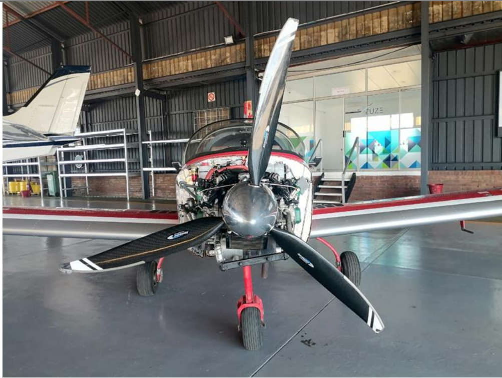
Figure 3: Damage to the propeller tips. (Source: Operator)
