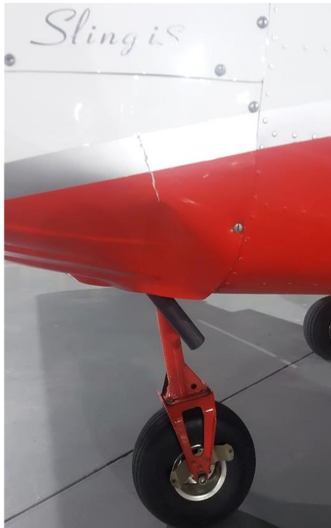
Figure 4: Damage to the nose gear. (Source: Operator)
