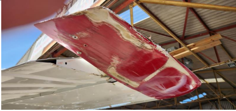
Figure 3: The damaged right-wing tip. (Source: Pilot)
