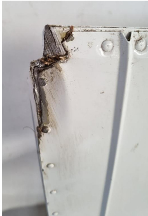
Figure 4: The damaged horizontal stabiliser. (Source: Pilot)
