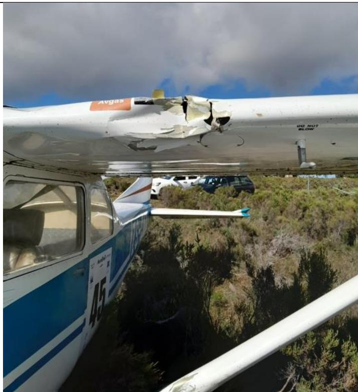
Figure 4: Damage sustained on the left-wing leading edge and strut. (Source: Operator)
