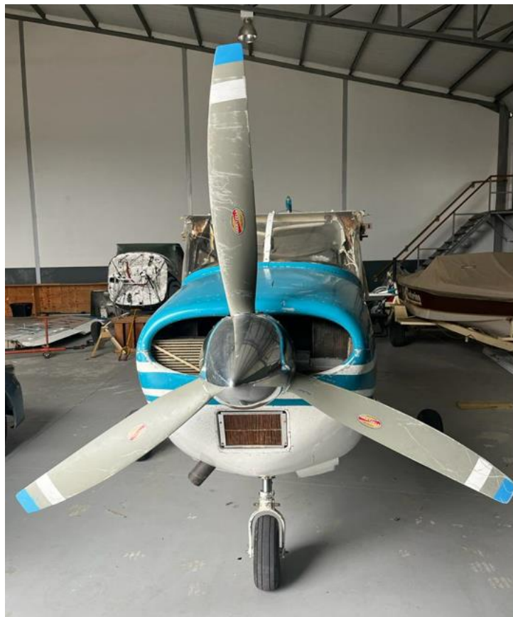
Figure 3: The scratch marks on the propeller blades due to impact with the fence.
