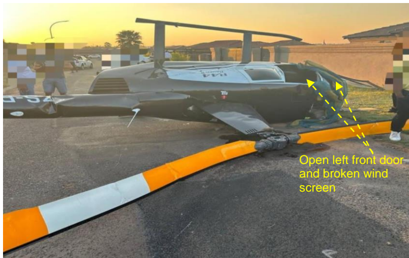
Figure 3: The open right front door and a broken wind screen. (Source: Operator)
