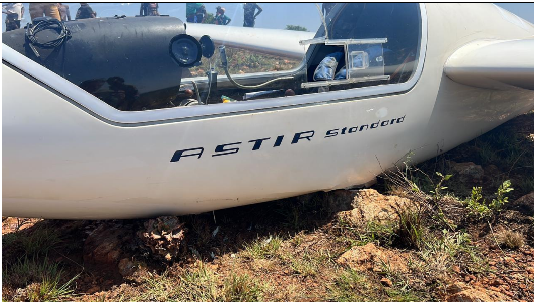
Figure 5: A closer view of the lower fuselage showing damage caused by the rocks. (Source: Pilot)
