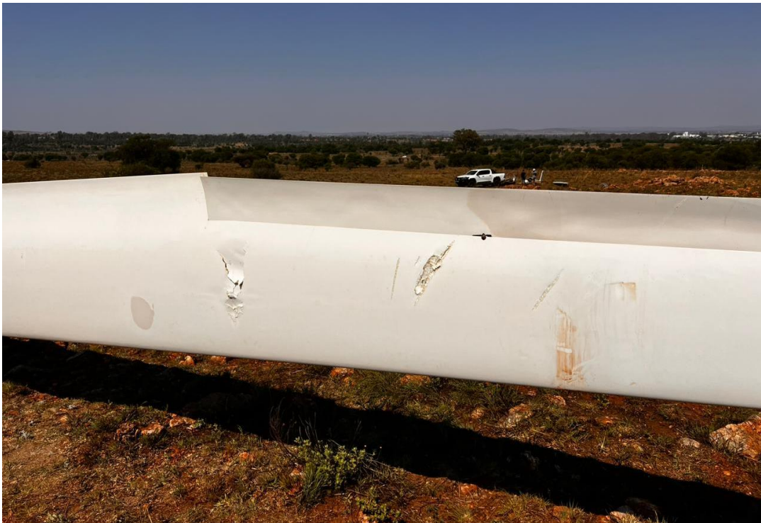
Figure 4: Damage to the right wing. (Source: Pilot)
