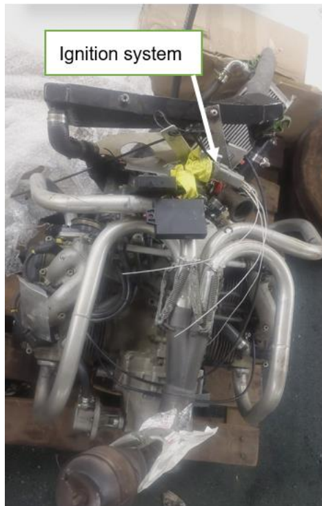
Figure 11: An unauthorised modification found on the ignition system.
