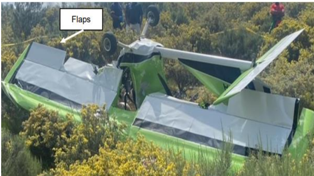
Figure 6: The damaged wings.
