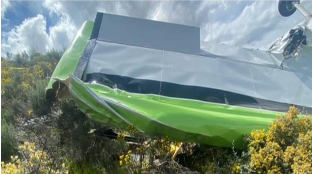
Figure 5: The damaged right-wing tip.
