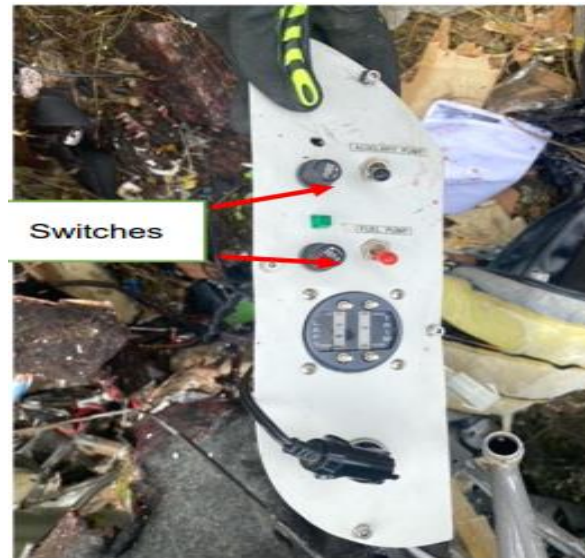
Figure 7: Auxiliary and fuel pump switches in OFF positions (red arrows).
