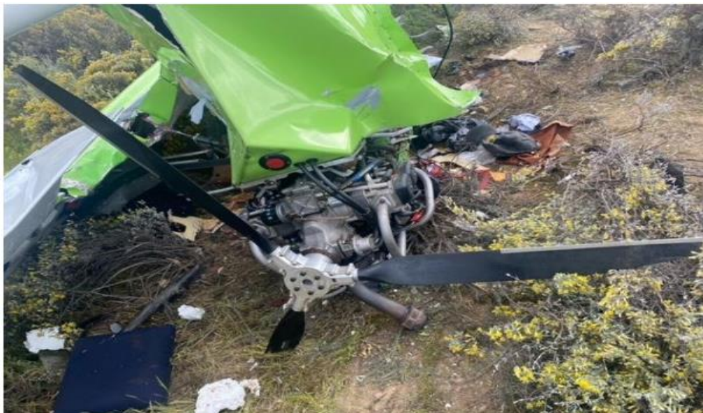
Figure 8: The damaged engine and propeller.
