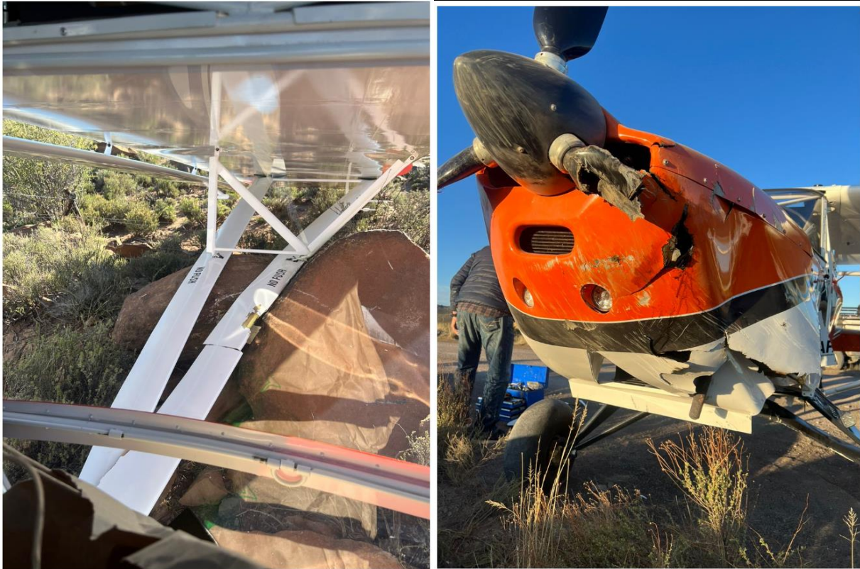
Figures 3 and 4: Damage to the left-wing support structure (left) and the engine cowling and propeller blades (in a coarse pitch position) (right). (Source: ARCC)
