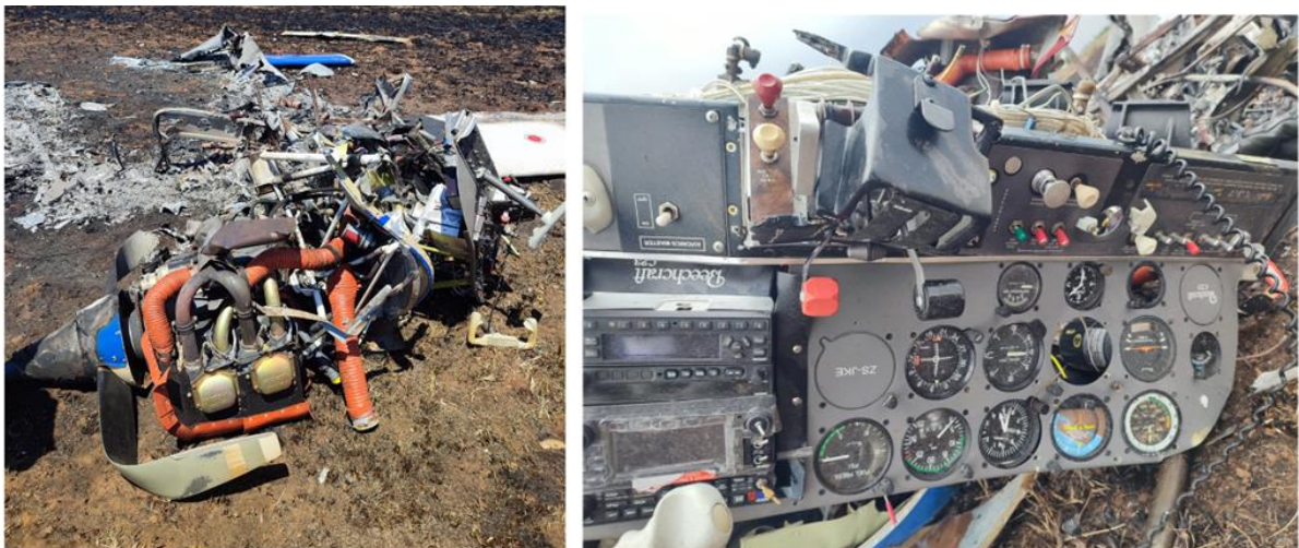
Figures 8 and 9: The damaged engine and propeller (left), and instrument panel (right).
