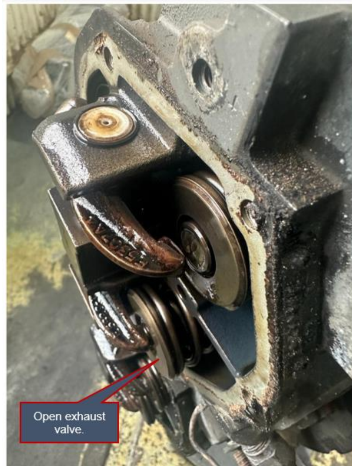
Figure 12: Cylinder No 4 exhaust valve in open position.
