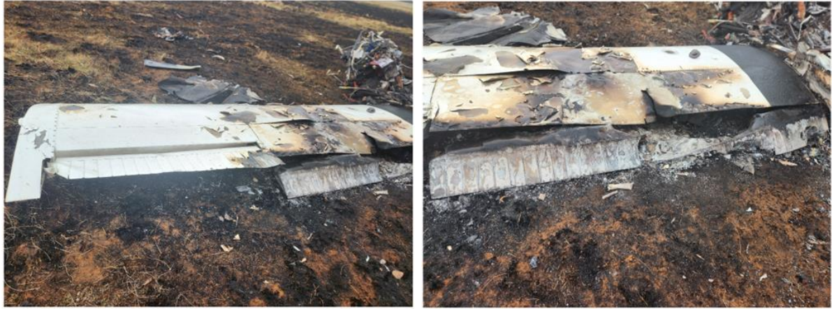
Figures 6 and 7: The damaged left aileron and flap (left). Closer-up picture of the left wing (right).
