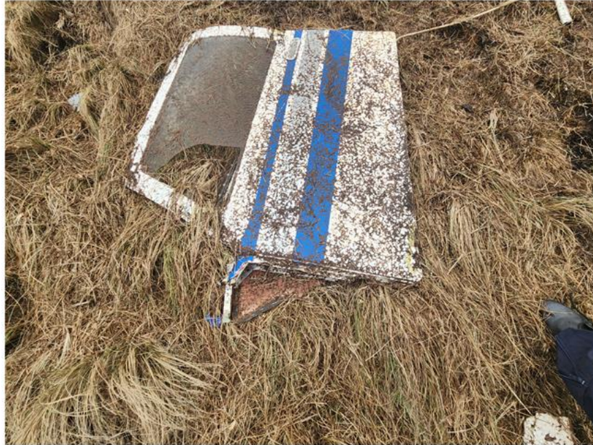
Figure 10: The left door that separated from the fuselage.
