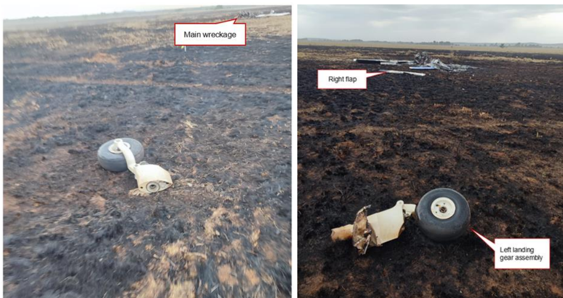
Figures 4 and 5: The right main landing gear assembly (left); and the left main landing gear assembly (right).
