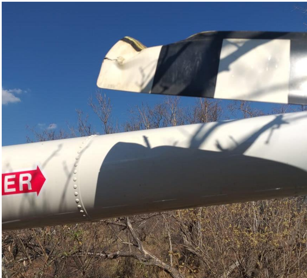
Figure 4: Damage to one of the tail rotor blades. (Source: Pilot)
