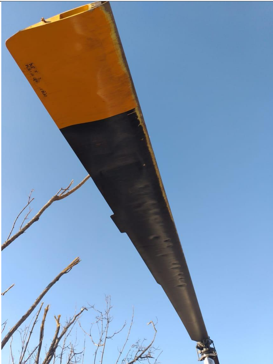
Figure 5: Damage to one of the main rotor blades. (Source: Pilot)
