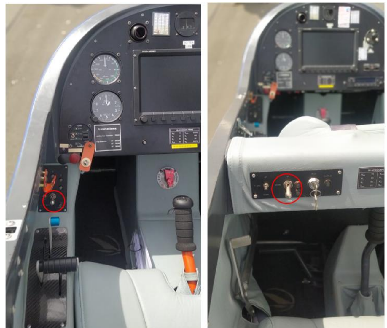
Figures 3 and 4: Red circles indicate front and rear cockpit control switches. (Source: Operator)
