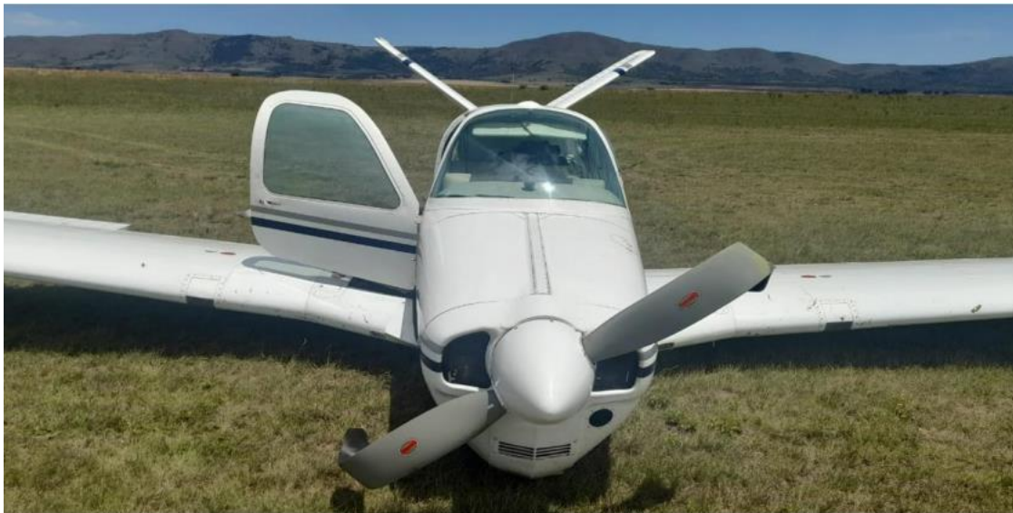
Figure 1: The damaged propeller blades. (Source: Operator)
