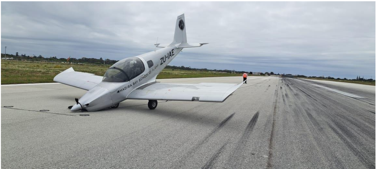
Figure 2: All propeller blades were damaged, and the nose wheel bent backwards. (Source: Operator)
