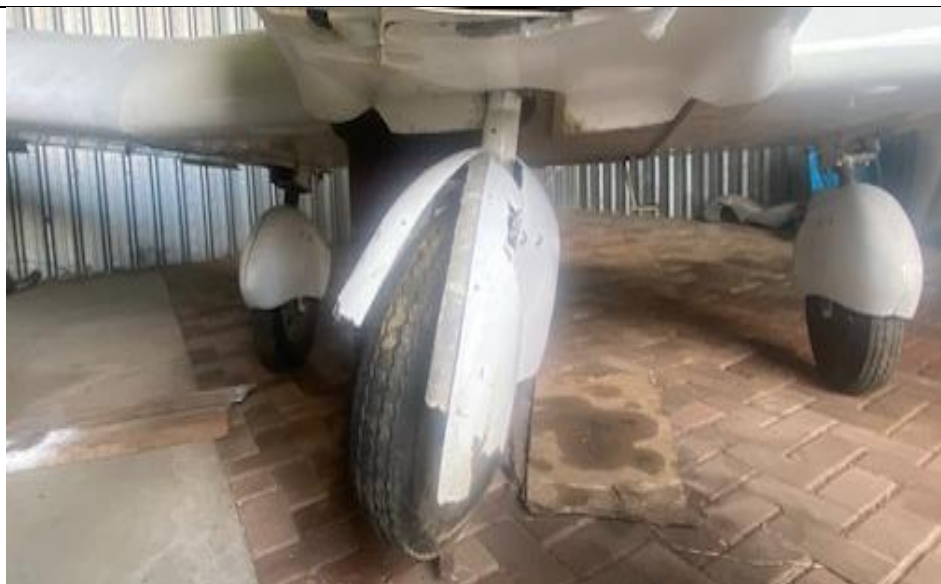
Figure 3: Bent nose gear strut and the damaged wheel fairing.
