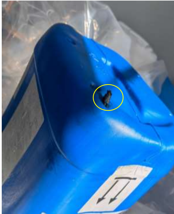
Figure 8: A DZUS fastener pierced through the bottom part of a chemical container.
