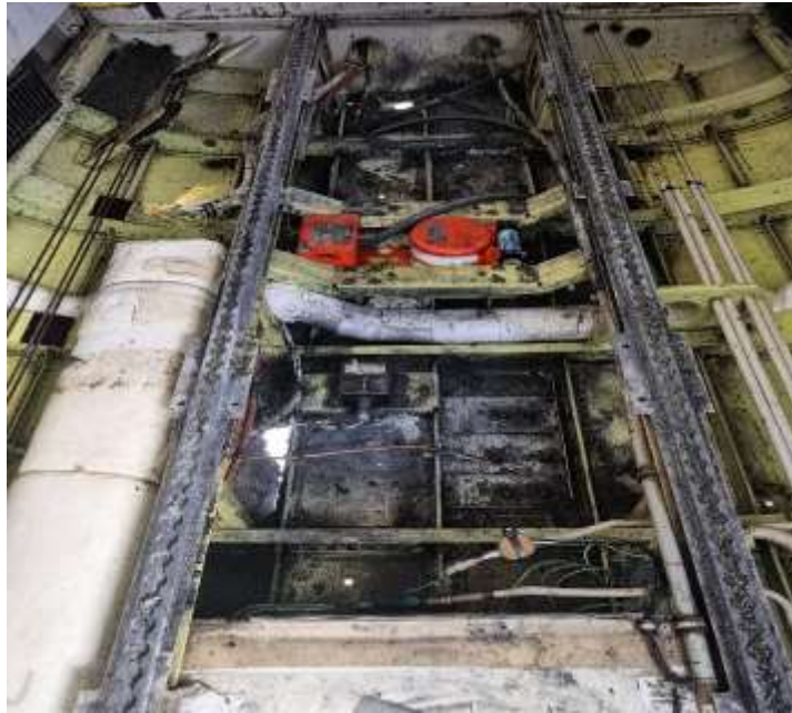
Figure 3: A closer view of the cabin area with evidence of damage on the under-fuselage skin caused by the corrosive chemical. (source: Operator)
