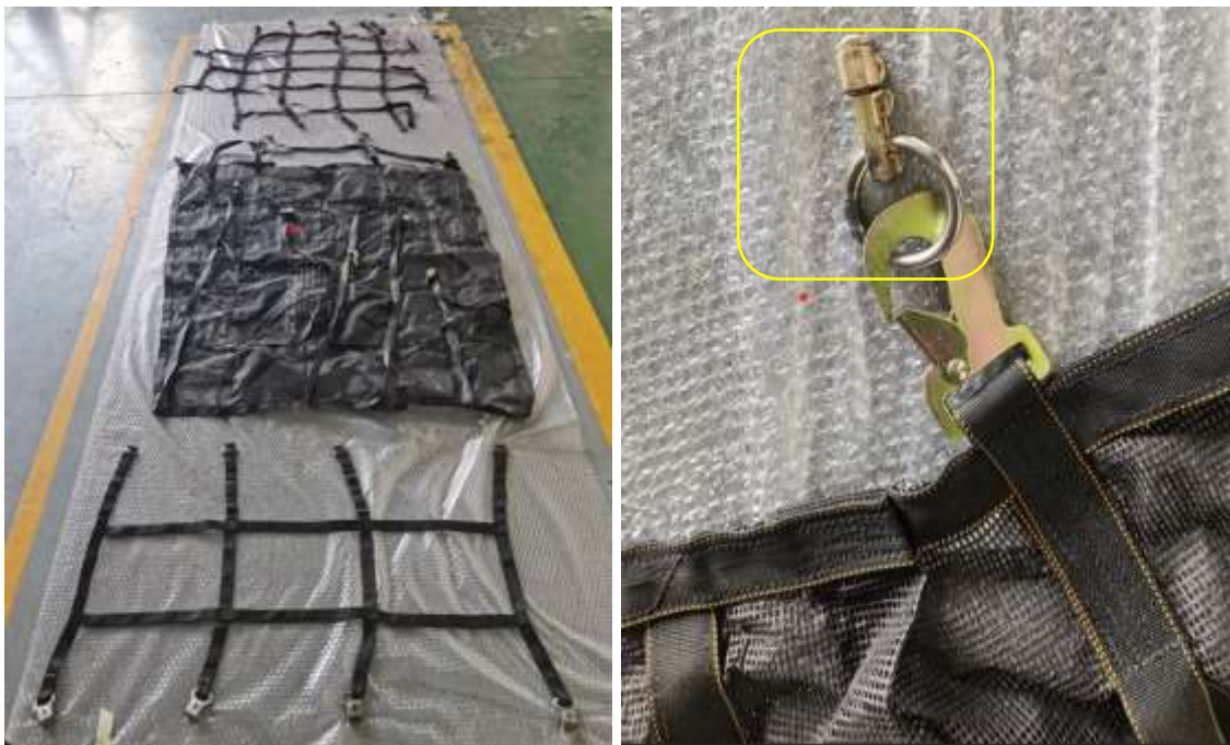
Figures 6 and 7: The net used to secure the cargo (left). The type of a lock that secured the cargo to the cabin floor rail.
