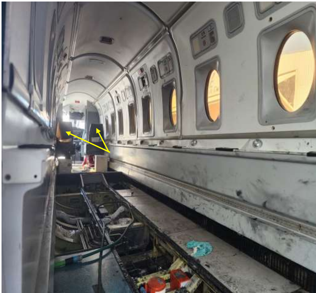
Figure 2: A picture showing the aircraft cabin with the floorboards removed to view damage. The yellow lines point to the two passenger seats behind the cockpit partitioning. (Source: Operator)
