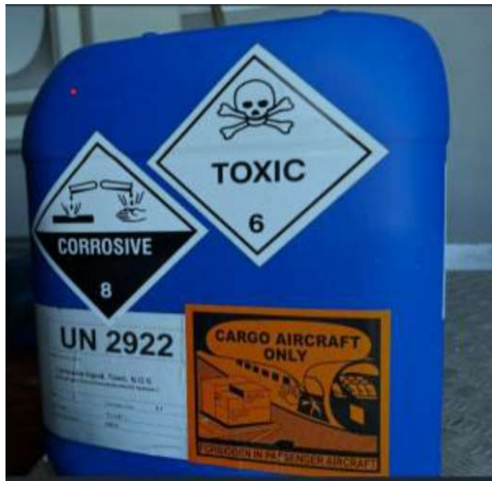
Figure 5: The 20l container with warning information. (Source: Operator)
