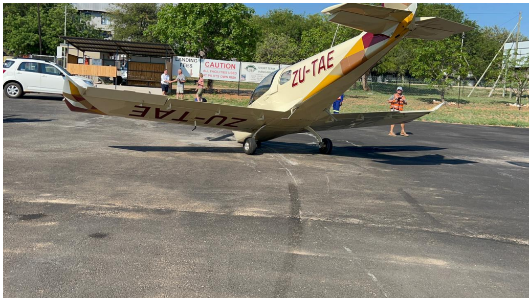
Figure 2: The aircraft with the collapsed nose gear after the accident.
