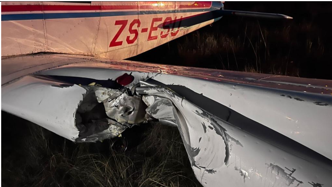
Figure 2: Damage to the left wing of the aircraft. (Source: Operator)
