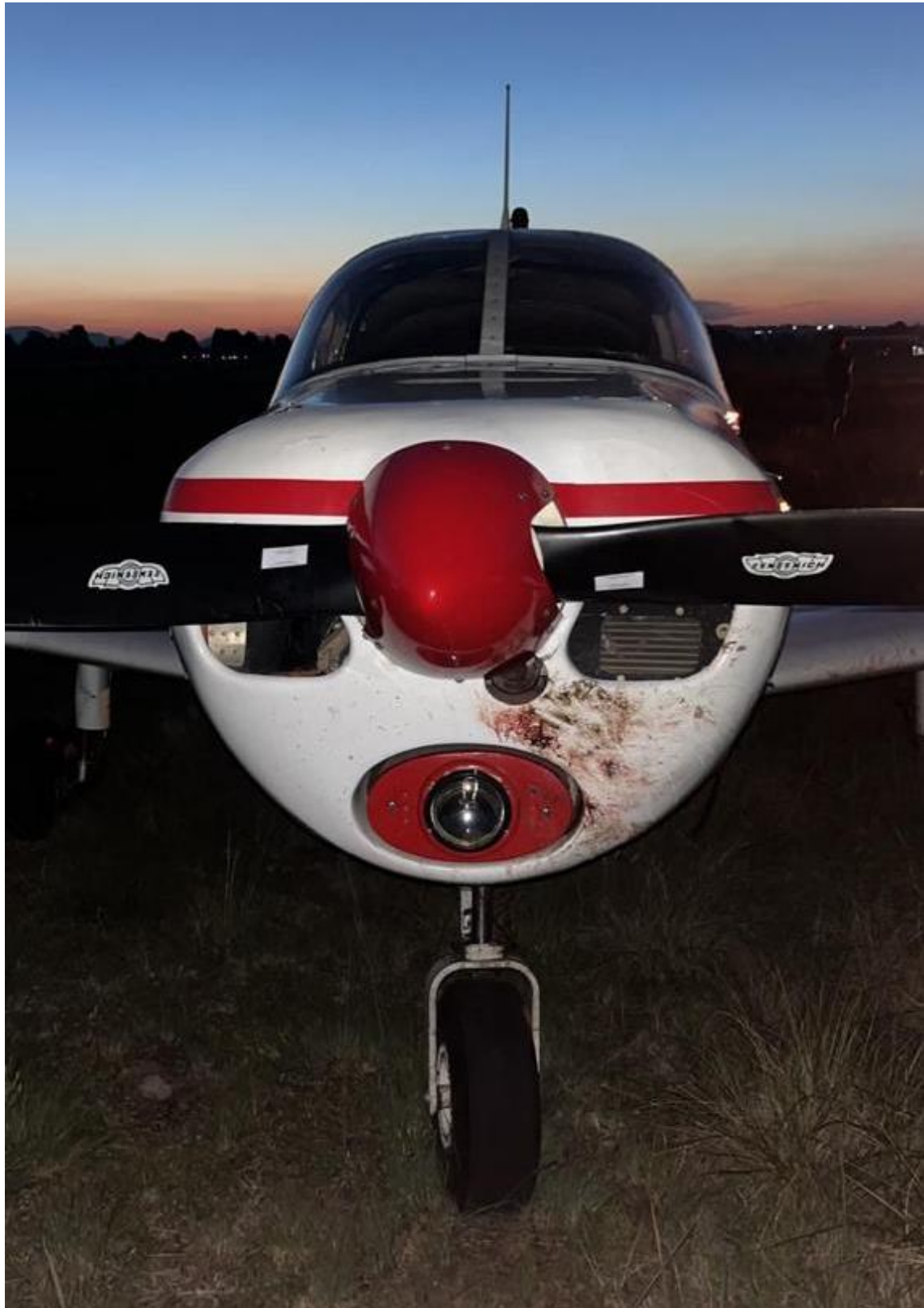
Figure 1: Bird strike mark on the aircraft. (Source: Operator)
