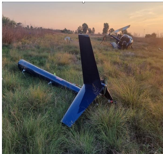
Figure 6: The main wreckage and the severed tail boom.
