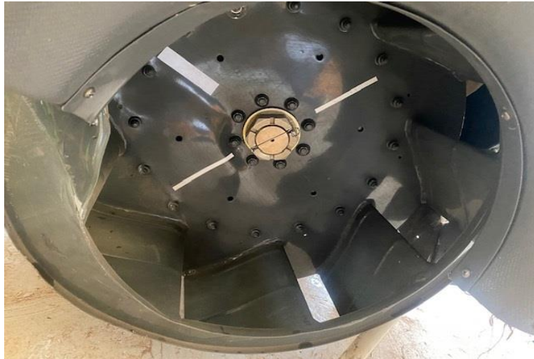
Figure 9: The engine cooling fan.
