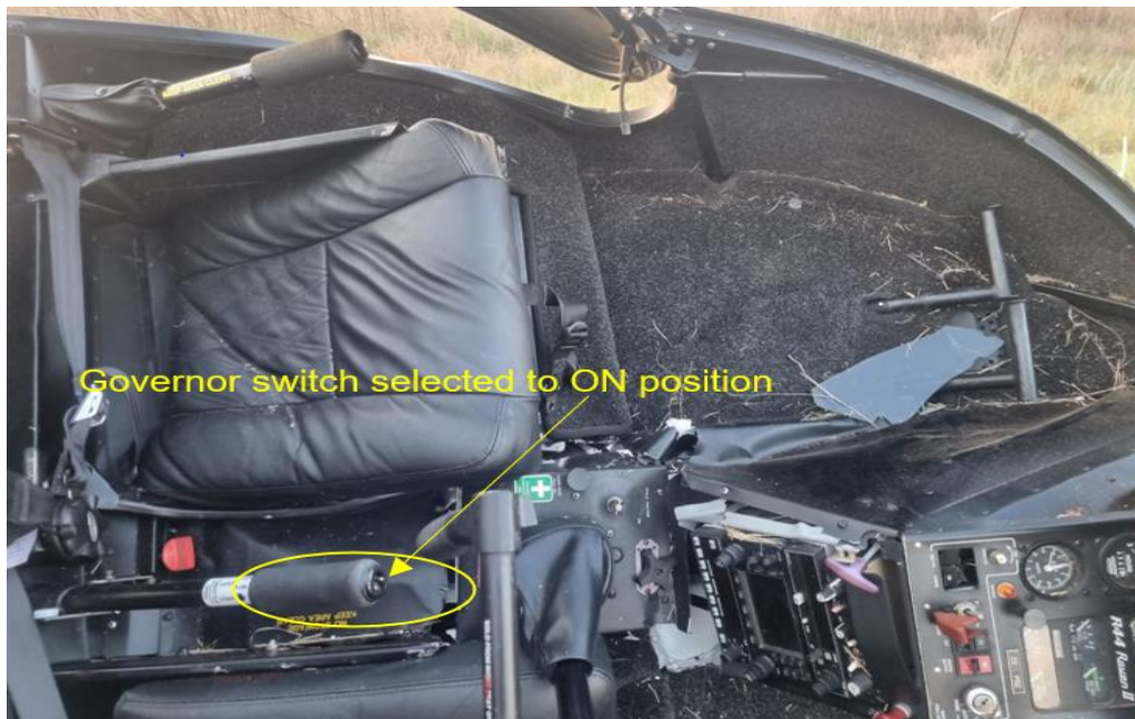
Figure 7: The pilot's collective pitch control stick in the UP position and the governor switch in the ON position.
