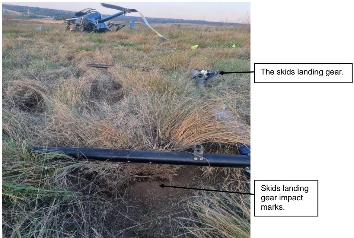
Figure 5: The wreckage and the broken skids landing gear.
