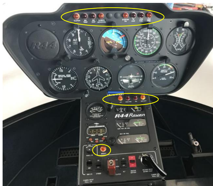
Figure 4: The Robinson R44, Raven II instrument panel showing warning lights.
