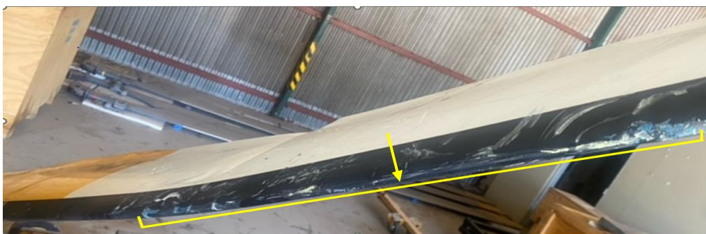
Figure 8: The main rotor blade leading edge area showing the impact print.
