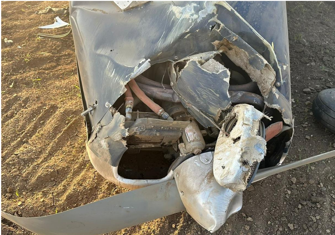
Figure 5: Damage to the nose cone.
