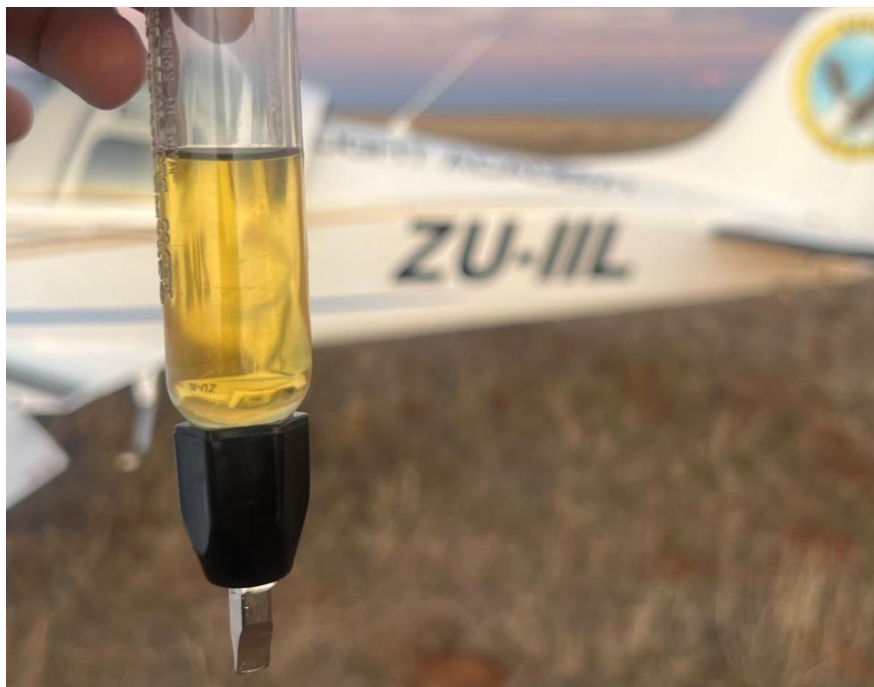
Figure 5: The fuel sample drained from the left-wing port. (Source: Operator)
