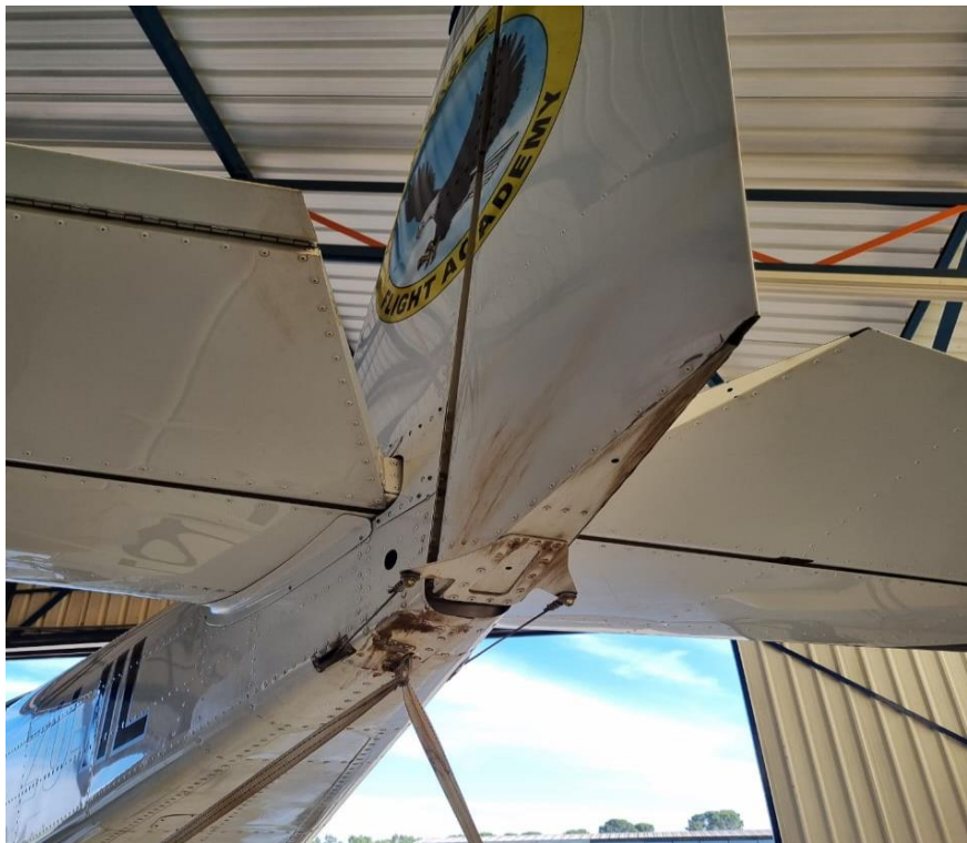
Figure 3: Scrape marks on the under skin of the tail section. (Source: Pilot)
