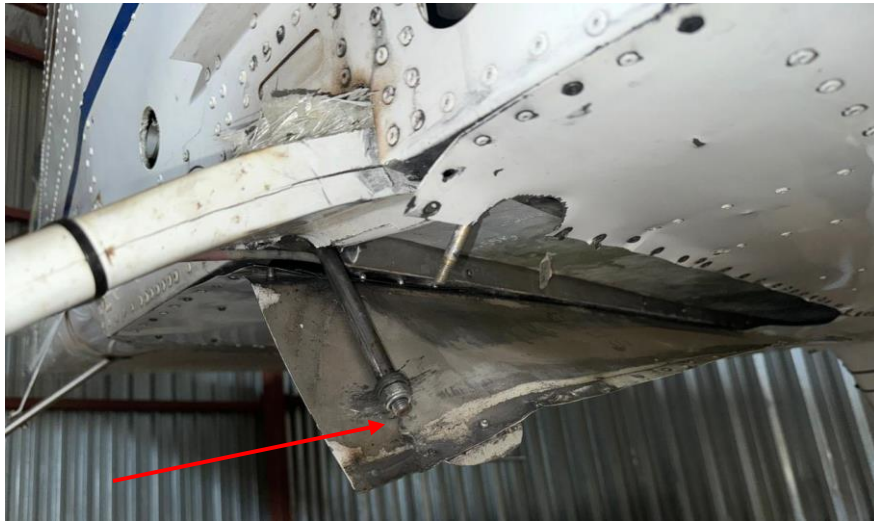
Figure 4: The landing gear attachment bolt that dislodged from the landing gear assembly and the damaged landing gear strut. (Source: Operator)
