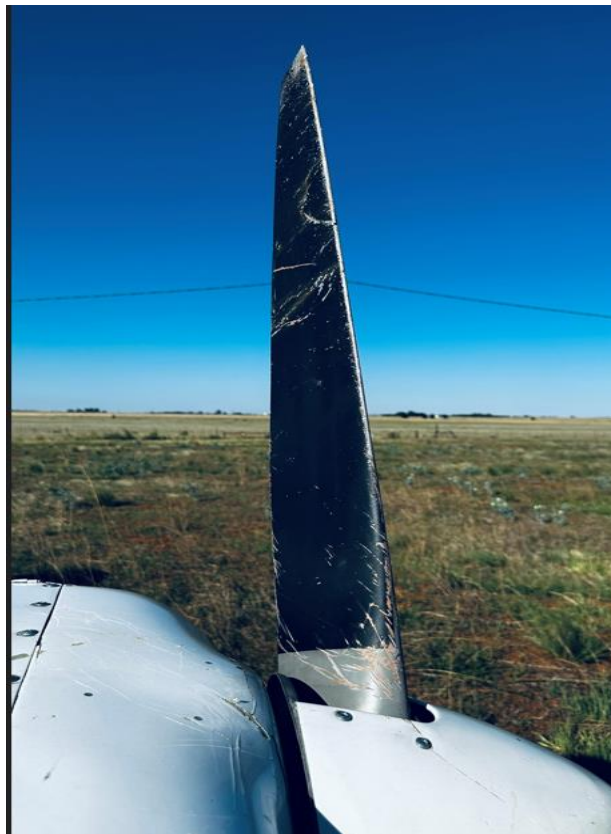
Figure 3: The propeller blade with scratch marks. (Source: Operator)
