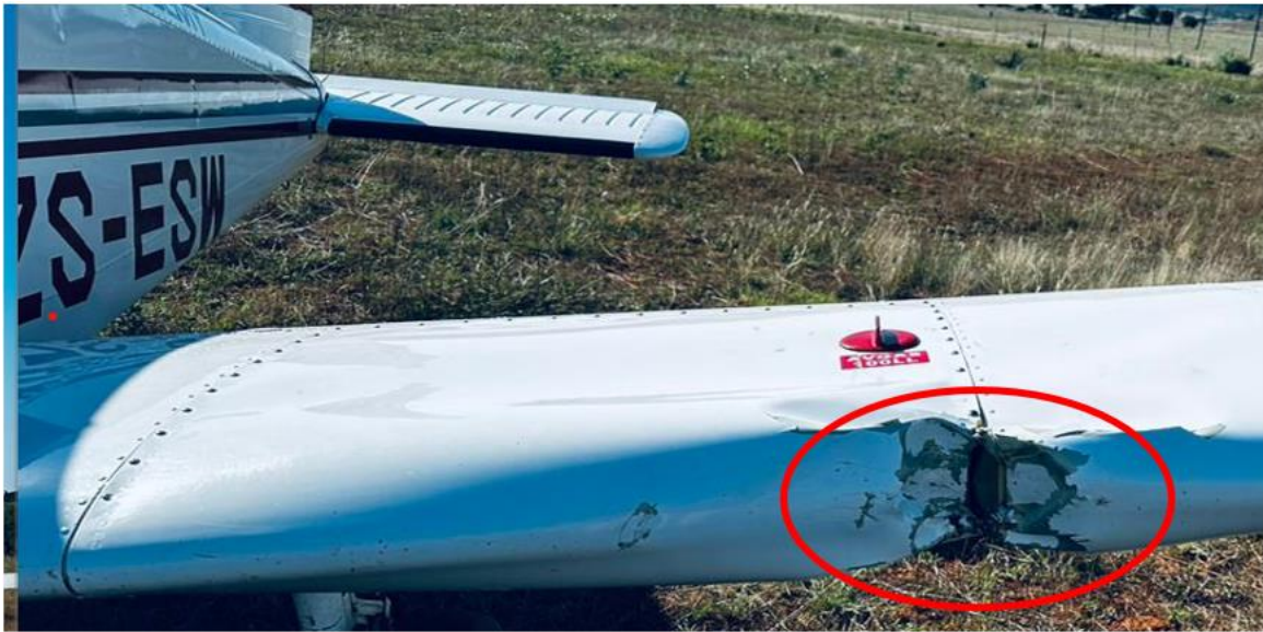
Figure 1: The dented left-wing leading edge. (Source: Operator)
