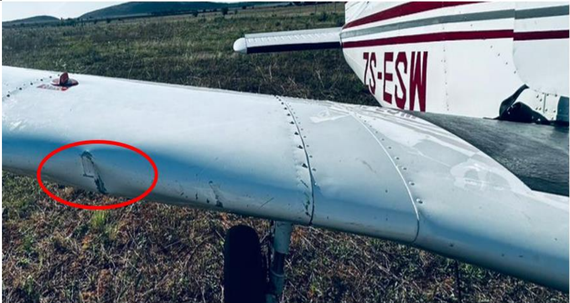
Figure 2: The dented right-wing leading edge. (Source: Operator)
