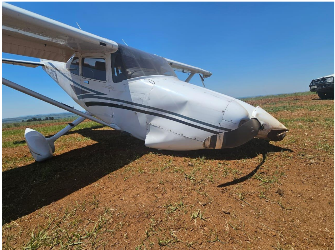
Figure 3: A closer view of the damage to the propeller and the lower fuselage. (Source: Pilot)
