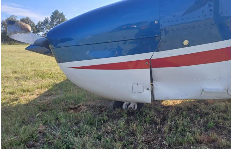
Figure 2: The damaged nose gear. (Source: Operator)
