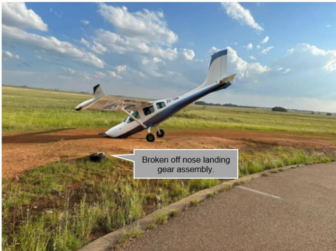
Figure 2: The aircraft as it came to rest on the right side of Runway 09 near the threshold of RWY 27. The nose gear strut that broke off is in the foreground. (Source: Pilot)
