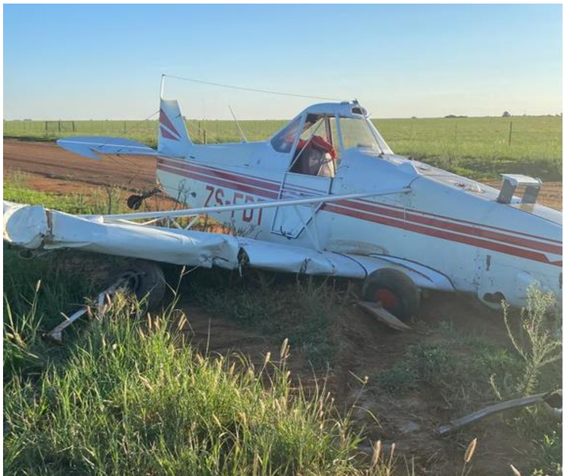
Figure 3: Damage on the right side of the aircraft and the severed undercarriage.
