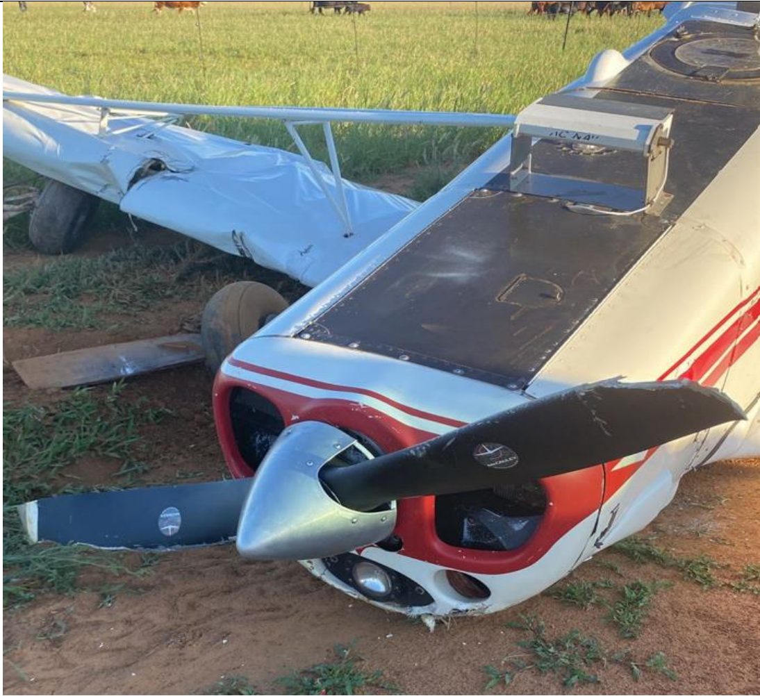
Figure 4: Damage to the propeller and the right wing.
