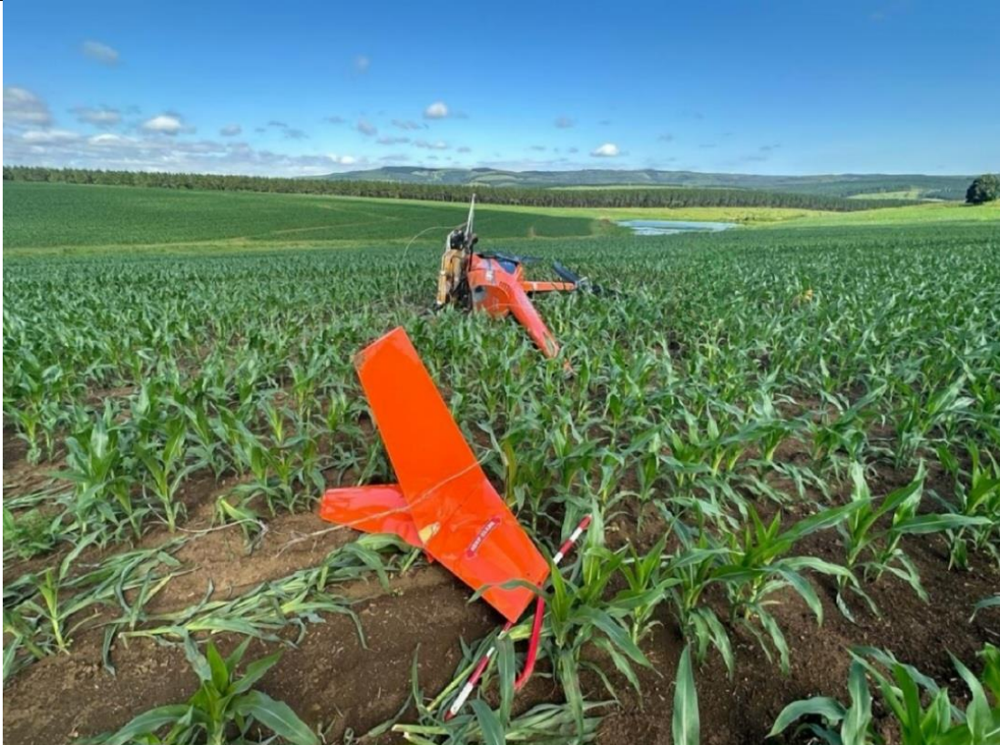
Figure 3: The severed tail rotor at the accident site. (Source: Operator)
