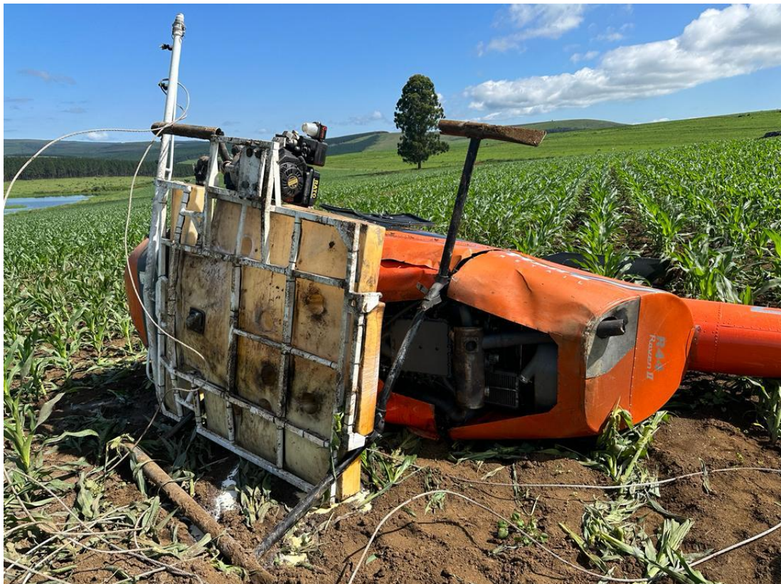
Figure 4: Damaged skids, spray boom and fuselage. (Source: Operator)
