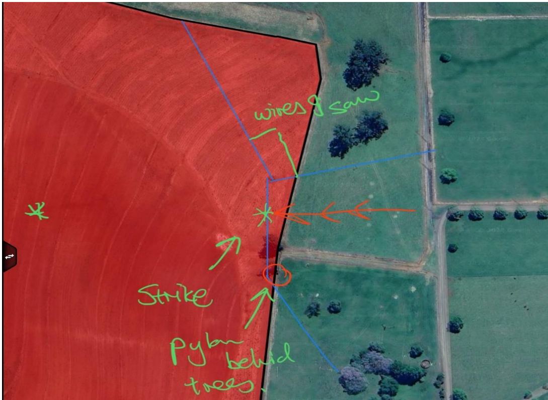
Figure 1: Sketch of the accident site. (Source: Pitot)
