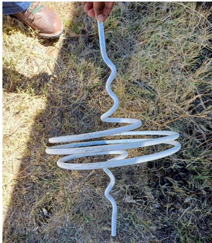
Figure 5: A bird diverter. (Source: Pilot)
