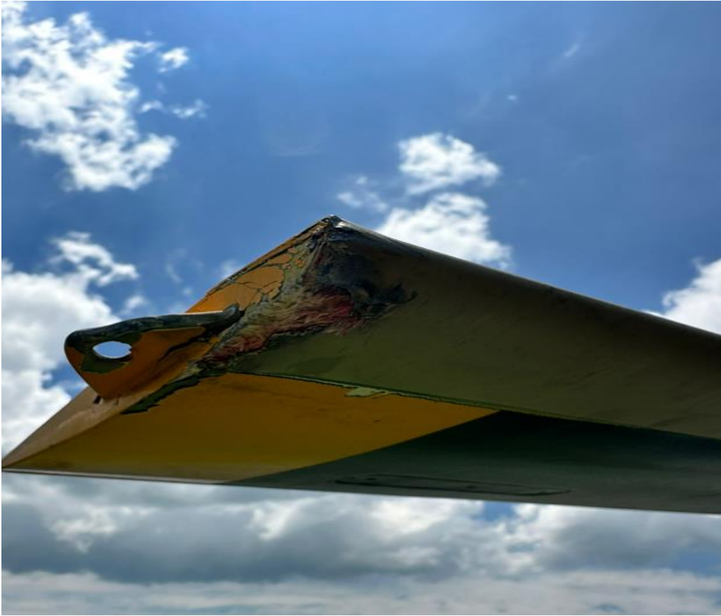
Figure 4: The damaged rotor blade. (Source: Pilot)
