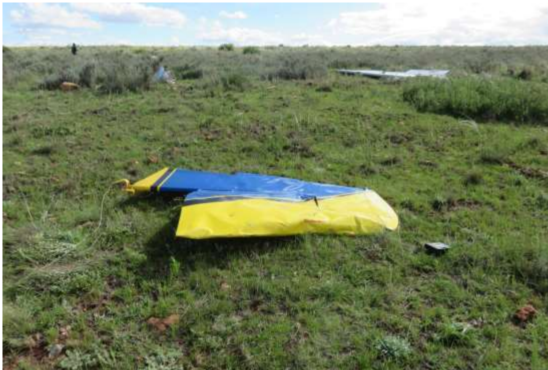
Figure 9: The vertical stabiliser and rudder assembly near the left wing of ZS-STD.
