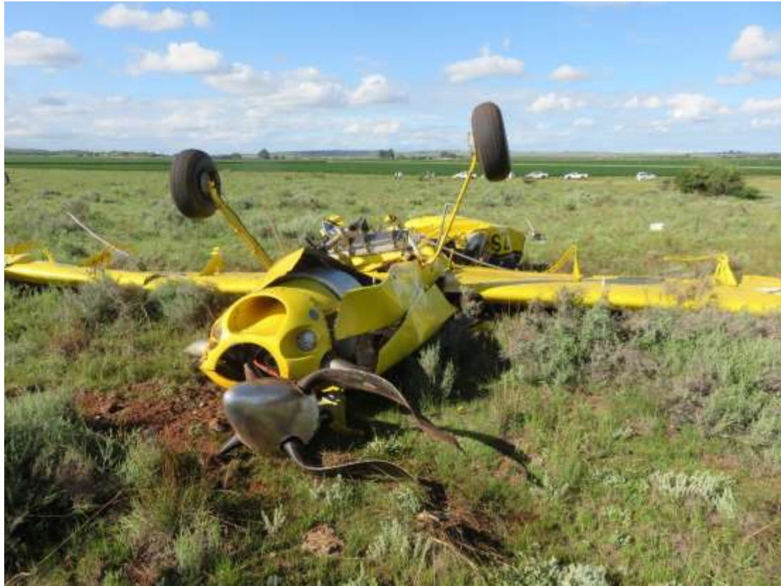
Figure 8: Deformed propeller blades, with one broken off.
