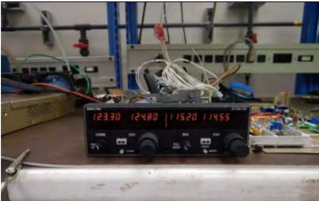
Figure 14: Radio frequencies displayed during testing. (Source: Honeywell)
