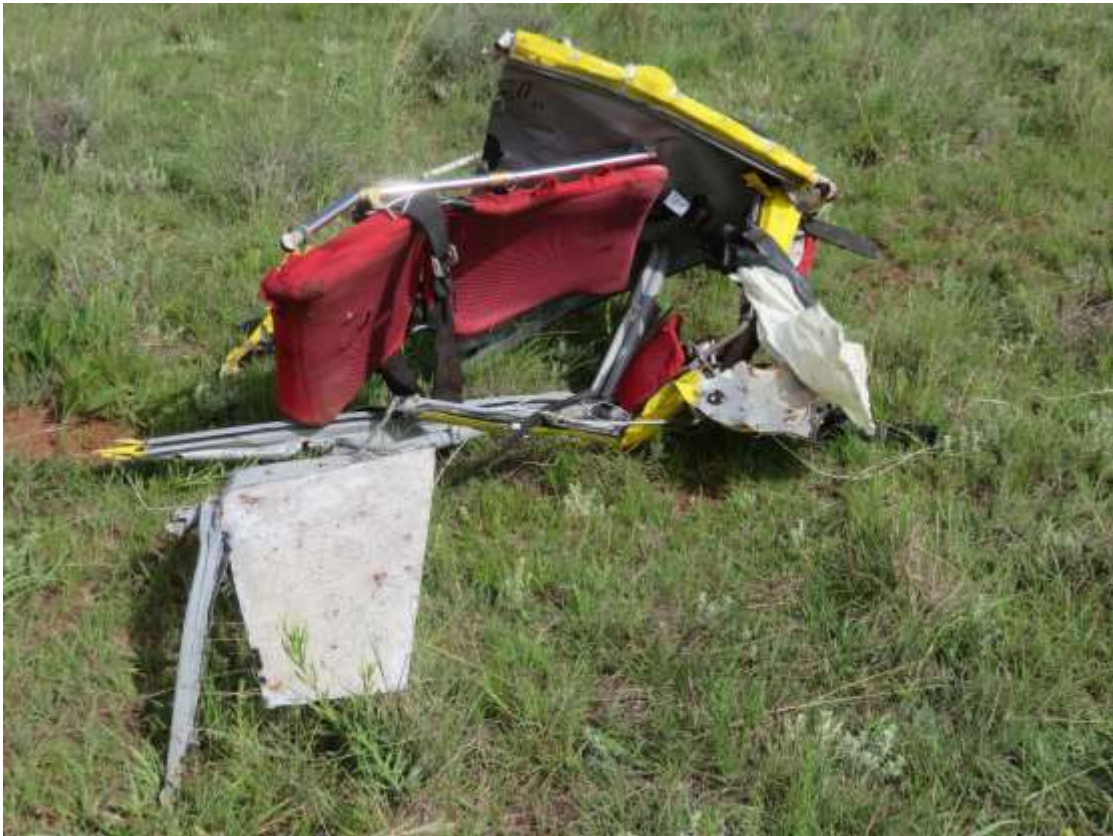
Figure 11: The pilot's seat and floor structure of ZS-XPC.
