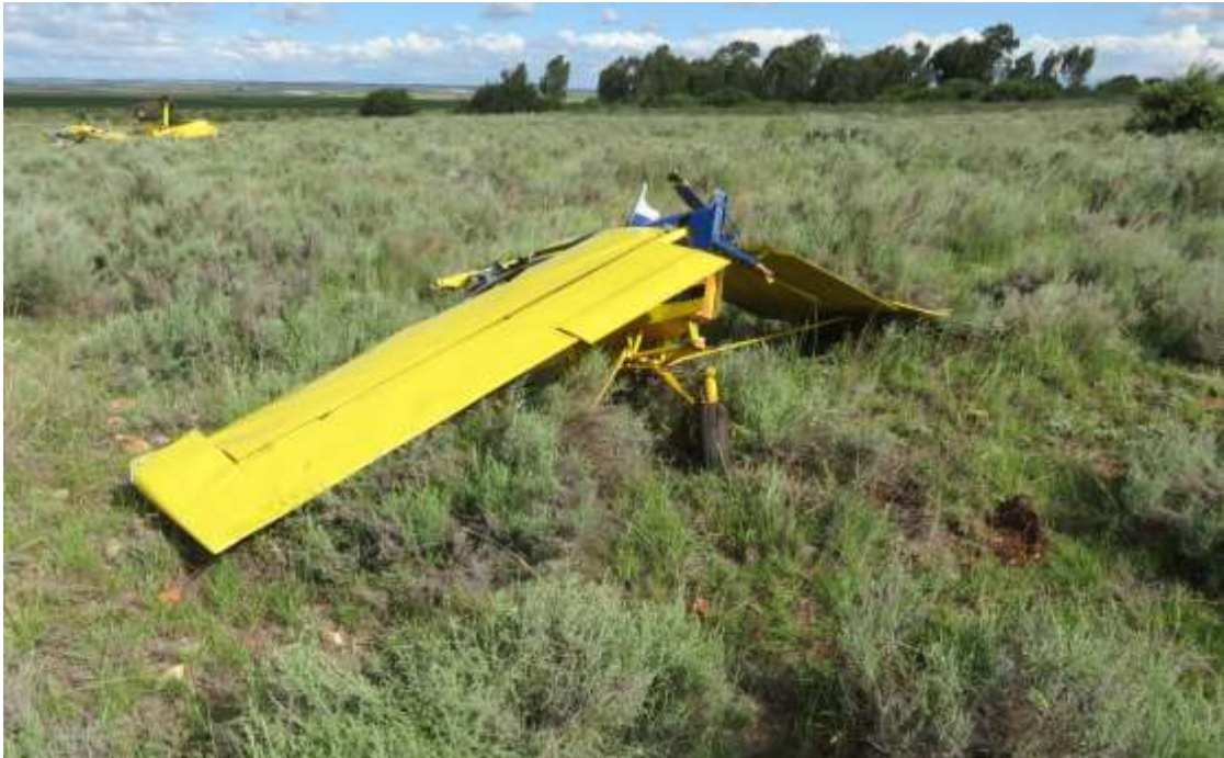
Figure 10: The aft fuselage and empennage with the two horizontal stabilisers still attached.
